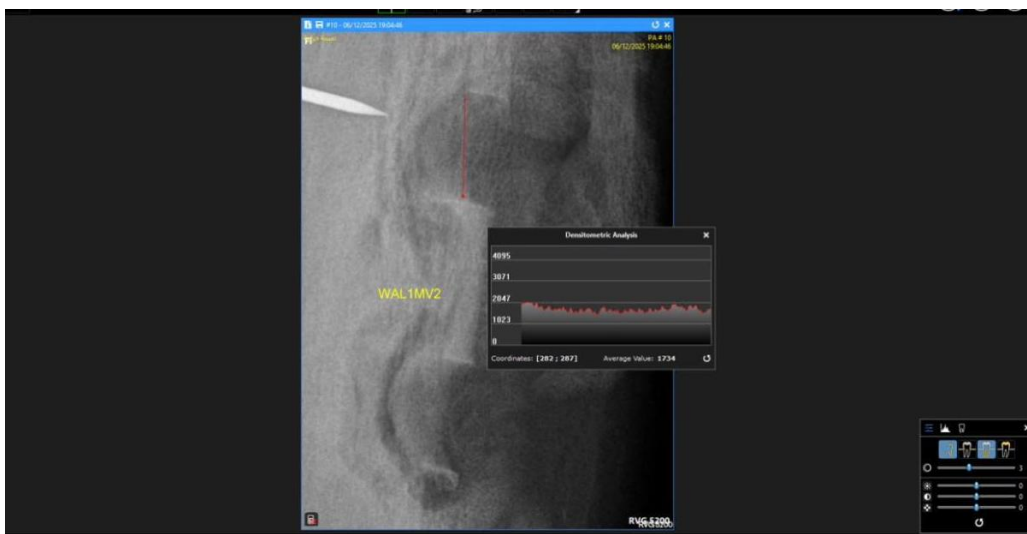
Fig. 5. Radiographic densitometric screenshot labelled WAL1MV2, showing the measured region around the defect site with an average value of approximately 1734.
