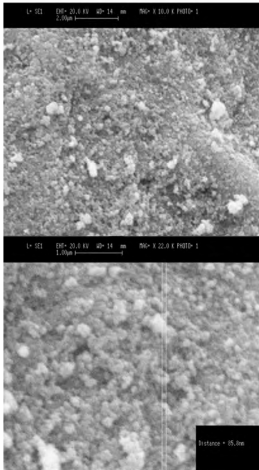
Fig. 4. SEM images of ZnO nanoparticles
