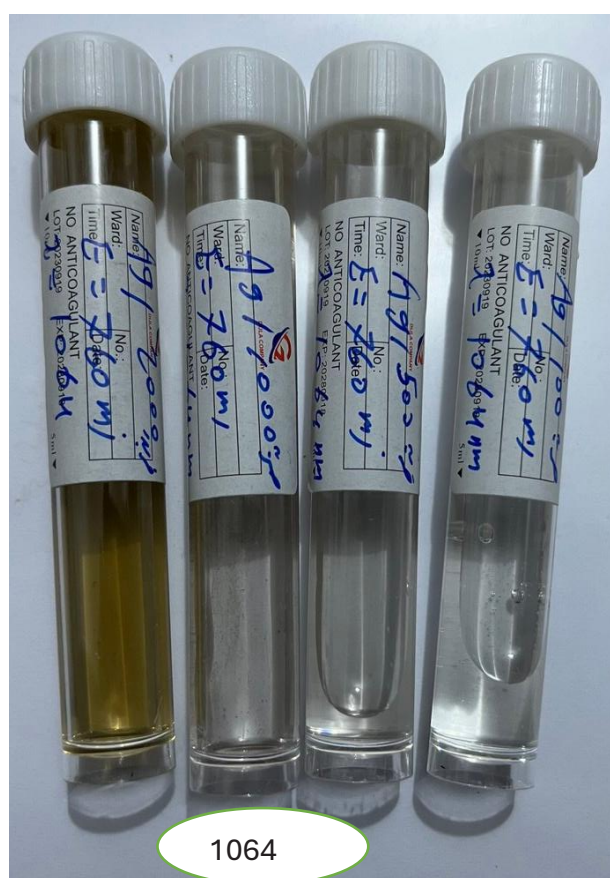
Fig. 2. Silver colour solution gradient at different pulse numbers of laser. solution obtained from silver metal using the PLAL method.
