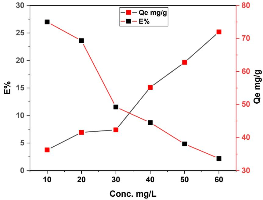
Fig. 6. Effect of the concentration of Cu (II) solution by using activated carbon Micro/Nano surface.
