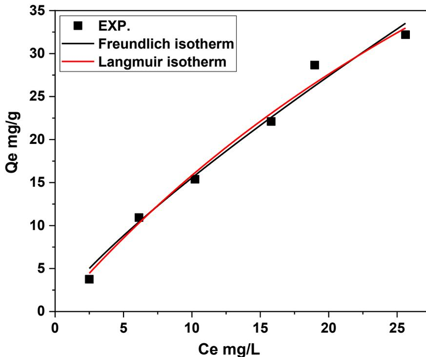
Fig. 8. Adsorption isotherm Freundlich model, and Langmuir model for Copper ions on the activated carbon Micro/Nano surface.
