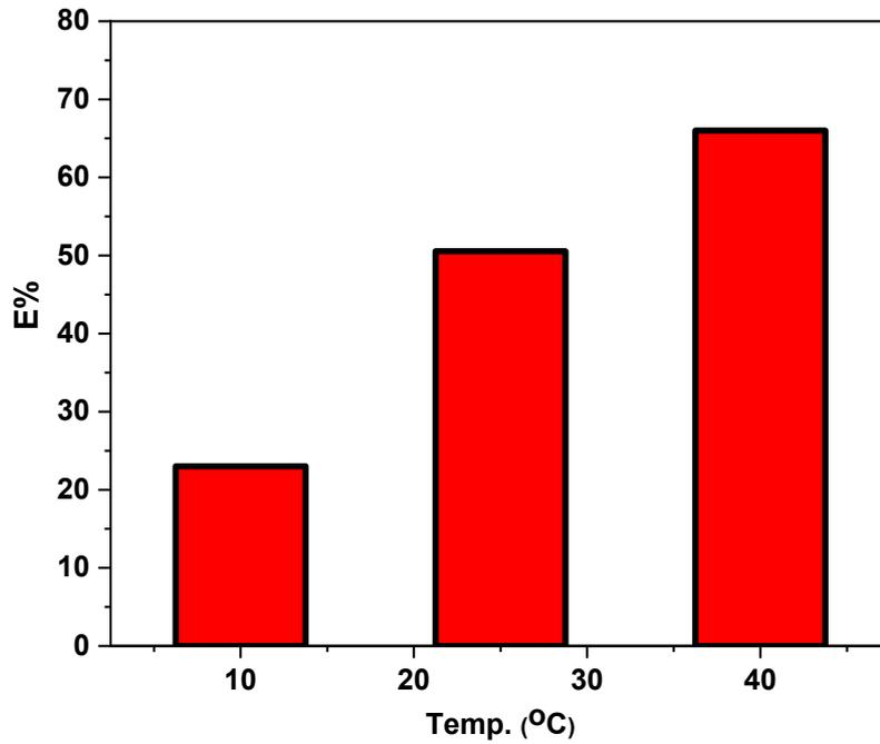
Fig. 7. Effect of Temperature solution on the removal of Cu(II) ions by activated carbon Micro/ Nano surface.
