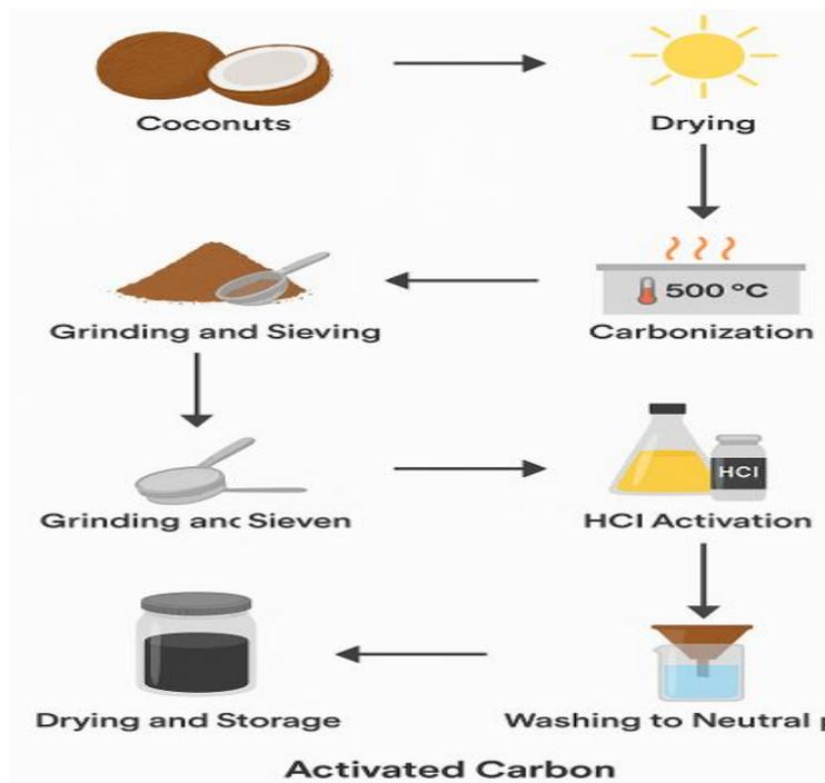
Fig. 1. Preparation of Hydrochloric Acid-Activated Carbon from Coconut Shells (AC-HCl).
