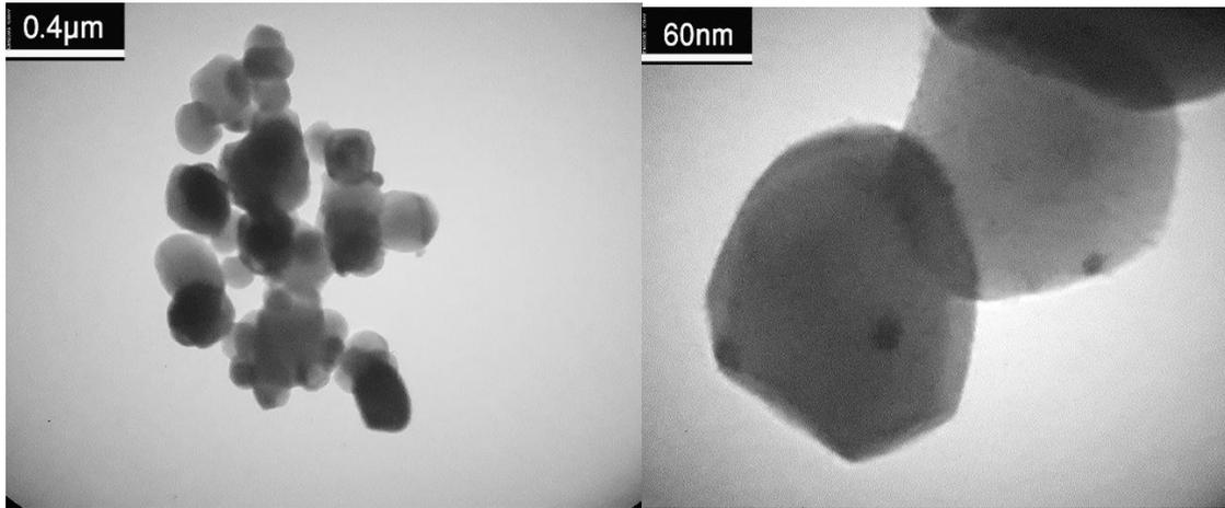
Fig. 4. TEM image of activated carbon Micro/Nano surface.
