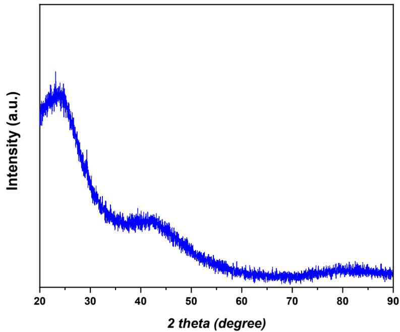
Fig. 2. X-ray diffraction (XRD) analysis of activated carbon Micro/Nano surface.
