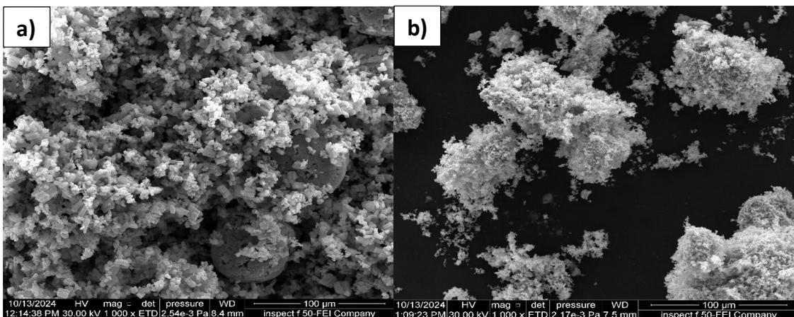
Fig. 3. ESEM image of a) activated carbon Micro/Nano surface before adsorption, b) after adsorption.
