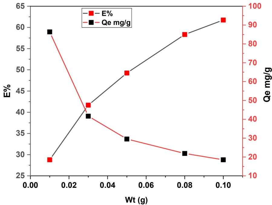
Fig. 5. Effect of the weight of the activated carbon Micro/Nano surface on the removal of Cu(II)ion.
