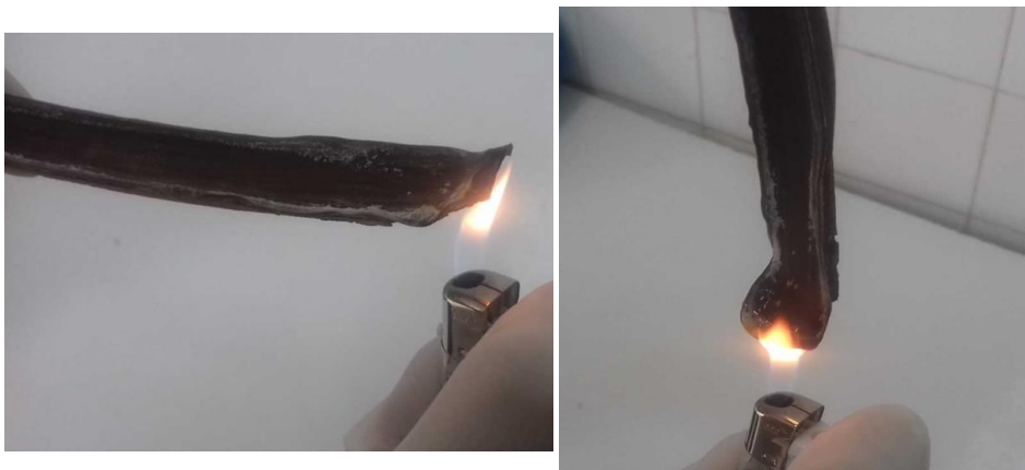
Fig. 11. PS-Fe 3 O 4 nanocomposite under UL-94 test
