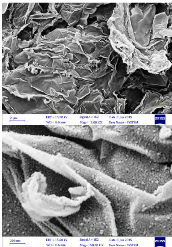
Fig. 7. SEM images of SiO 2 synthesized by oleic acid
