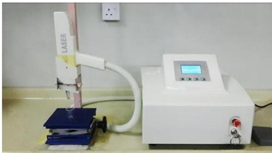
Fig. 1. The pulsed Nd-YAG laser system used in the work.
