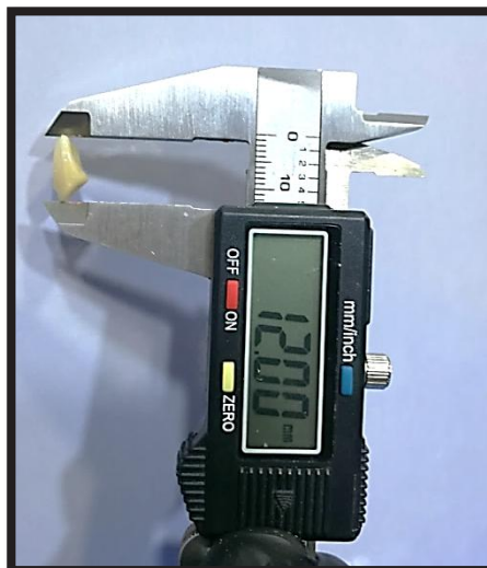
Fig. 2. The teeth were measured by used an electronic digital caliper
