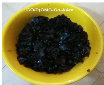
Fig. 2. Prepared GO/P(CMC-Co-Am) nanocomposite.
