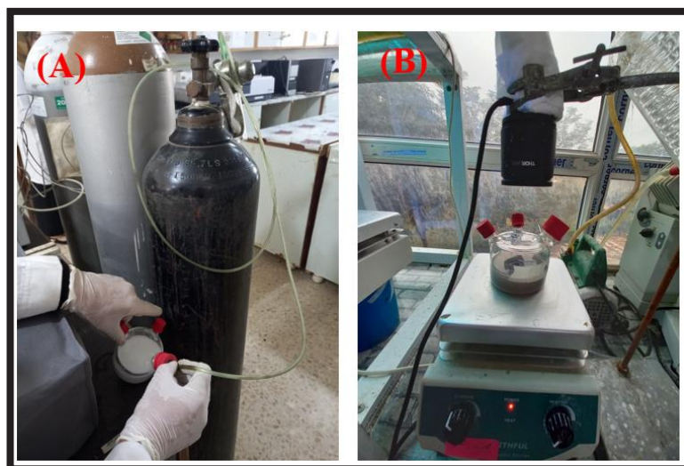
Fig. 2. Real image for the photo deposition of silver doped TiO 2 (A) purgulate the mixed surface to nitrogen gas (B) Irradiate the mixture with lamp LED.
