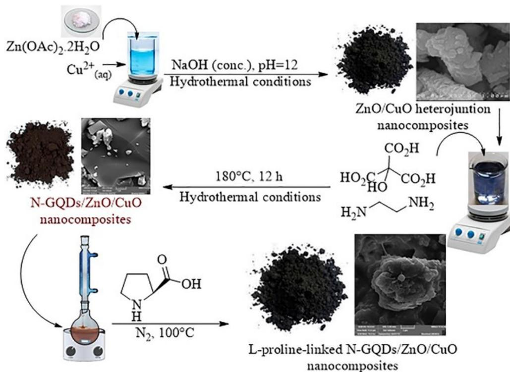
Fig. 2. Schematic procedure of L-proline-linked N-GQDs/ZnO/CuO nanocomposites.
