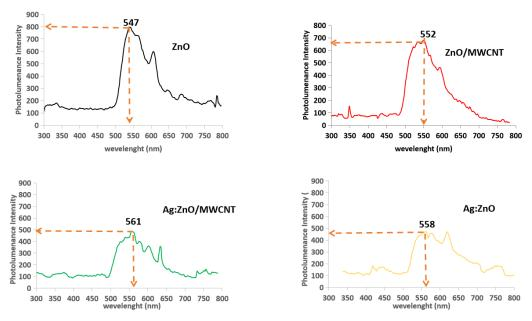
Fig. 2. Photo-luminescence (PL) spectra of ZnO, ZnO/MWCNT, Ag:ZnO and Ag:ZnO/MWCNT
