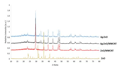
Fig. 1. XRD patterns for ZnO, ZnO/MWCNT, Ag:ZnO and Ag:ZnO/MWCNT
