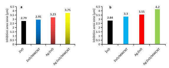
Fig. 3. the inhibition area zone of Acinetobacter baumannii by ZnO, ZnO/MWCNT, Ag:ZnO and Ag:ZnO/MWCNT (a) without irradiation , and (b) with irradiation with UV-A light (0.7 m W)
