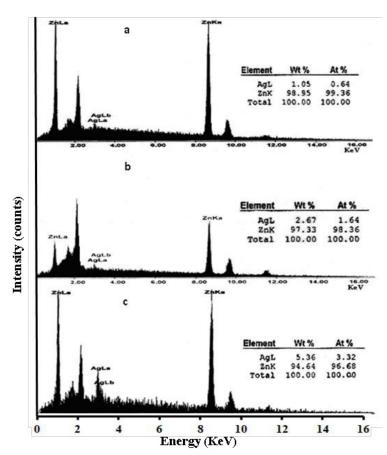
Fig. 2. EDS diagrams of the Ag/ZnO nanocomposites with different Ag loadings: (a) 1%Ag/ZnO (b) 2.5%Ag/ZnO (c) 5%Ag/ZnO.
