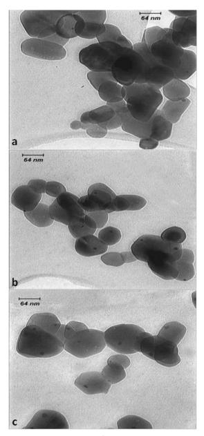
Fig. 3. TEM images of the Ag/ZnO nanocomposites with different Ag loadings: (a) 1%Ag/ZnO (b) 2.5%Ag/ZnO (c) 5%Ag/ZnO.
