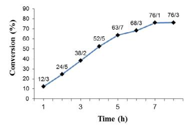
Fig. 4. The effect of reaction time on toluene conversion.
