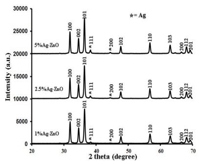
Fig. 1. XRD patterns of the Ag/ZnO nanocomposites with different Ag loadings.
