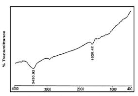
Fig. 1. Infrared spectra of MWCNTs treated with nitric acid.
