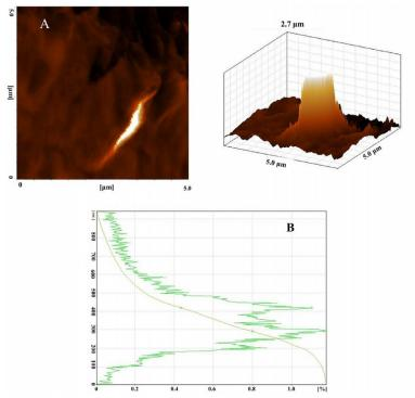
Fig. 7. (A) Typically AFM image of ss-DNA immobilization on MWCNT-COOH (image size: 5  $\mu$ m  $\times$  5  $\mu$ m  $\times$  2.7 $\mu$ m), (B) Image height distribution.
