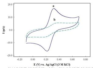
Fig. 3. Cyclic voltammograms of (a) MWCNT-COOH/GCE and (b) ss-DNA/MWCNT-COOH/GCE in presence of 0.01 M  $[Fe(CN)6]^{3\cdot/4}$  in 0.1 M KCl. Scan rate: 0.1 Vs<sup>-1</sup>.
