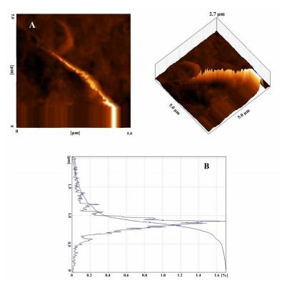
Fig. 6. (A) Typically AFM image of MWCNT-COOH (image size:  $5\mu m \times 5\mu m \times 2.7\mu m$ ), (B) Image height distribution.
