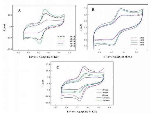
Fig. 5. Cyclic voltammograms recorded in presence of 0.01 M [Fe(CN)6] <sup>3-/4-</sup> containing 0.1 M KCl for ss-DNA immobilization on MWCNT-COOH/GCE as a function of (A) pH, (B) NaCl concentration and (C) incubation time.
