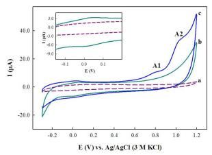
Fig. 2. Cyclic voltammograms of the modified GCE recorded in PBS (pH 7.0) at a scan rate of  $0.1~Vs^{-1}$ , in the potential range between -0.3 to +1.2 V (a) bare GCE, (b) MWCNT-COOH/GCE, and (c) ss-DNA/MWCNT-COOH/GCE.
