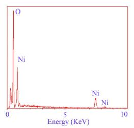
Fig. 9. EDS analysis of Ni(OH), nanoparticles
