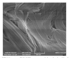
Fig. 2. SEM image of  $\rm Ni(OH)_2$  nanoparticles obtained by  $\rm NiSO_4-CTAB$
