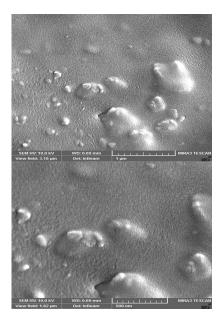
Fig. 7. SEM images of PVA-Ni(OH)<sub>2</sub> nanocomposite
