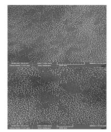
Fig. 3. SEM images of nanoparticles synthesized by  $NiNO_3$ -PEG
