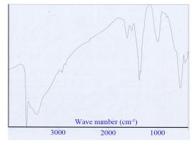
Fig. 8 FT-IR of Ni(OH), nanoparticles
