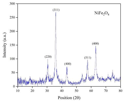
Fig. 1. XRD patterns of prepared  $NiFe_2O_4$  nanoparticles.
