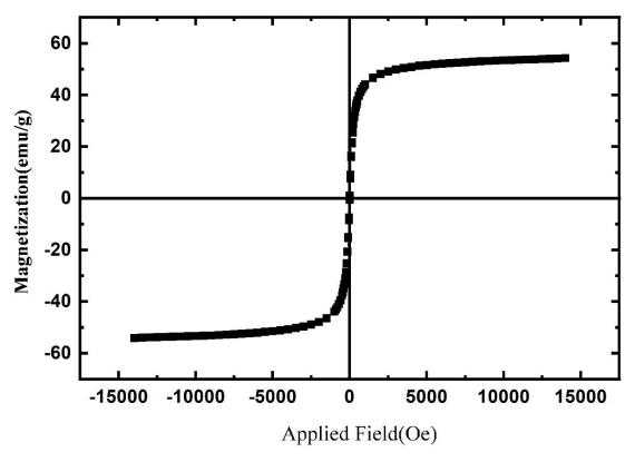
Fig. 5. VSM analysis of synthesized  $NiFe_2O_4$  nanoparticles
