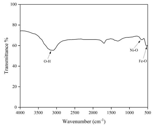
Fig. 2. FTIR spectrum of prepared NiFe<sub>2</sub>O<sub>4</sub> nanoparticles.
