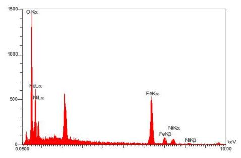
Fig. 4. EDS analysis of as-obtained NiFe<sub>2</sub>O<sub>4</sub> nanoparticles.
