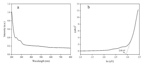
Fig. 6. a) UV-Vis absorption spectra of synthesized NiFe<sub>2</sub>O<sub>4</sub> nanoparticles b) Optical band gap of prepared NiFe<sub>2</sub>O<sub>4</sub> nanoparticles
