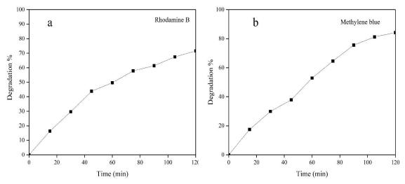
Fig. 7. Photocatalytic activity of prepared NiFe<sub>2</sub>O<sub>4</sub> nanoparticles against a) Rhodamine B b) Methylene blue under visible light.
