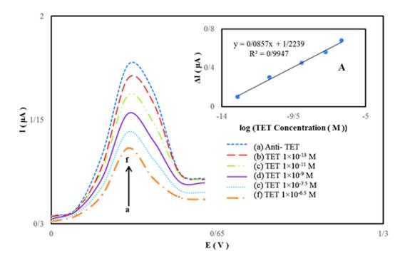
Fig S1. Voltammograms of Anti-TET/Pyr/Chi/GO/GCE aptasensor before (as a blank solution) and after hybridization with different concentrations of TCs (the number of repetitive experiments is six). Inset A: the dependence of  $\Delta I$  versus the concentration of target.
