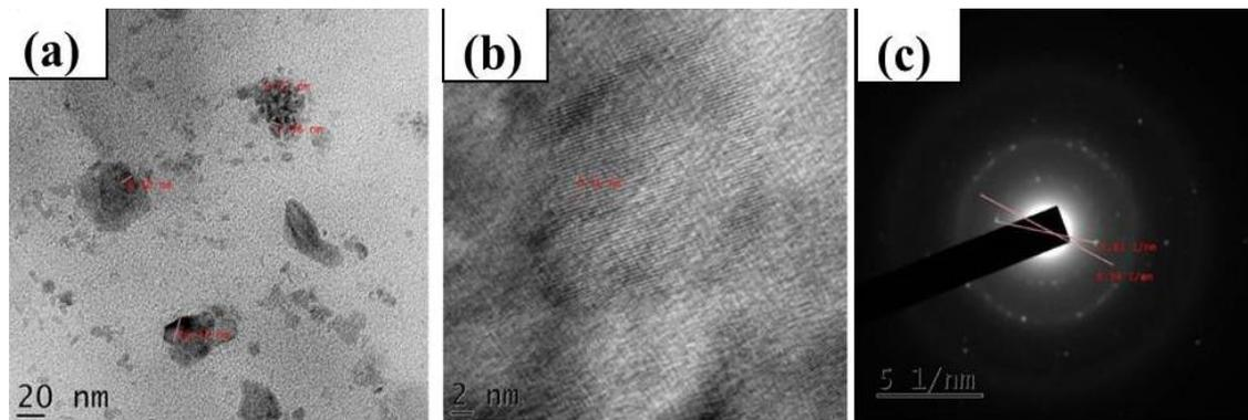
Fig.3. Image of Zinc copper ferrites nanoparticles annealed at 600°C, (a) HRTEM (b) Inter planar distance (c) SAED
