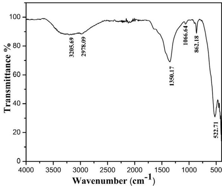
Fig.4. FT-IR spectra of Zinc copper ferrite nanoparticles.
