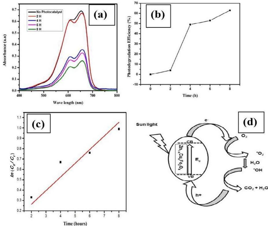
Fig.6. Zinc copper ferrite nanoparticles annealed at 600°C under UV-light irradiation (a) Absorption of MB solution during the photo-degradation (b) Photo-degradation percentage (c) Plots of  $\ln(C_0/C_t)$  versus irradiation time (d) Photocatalytic mechanism of MB in catalyst.
