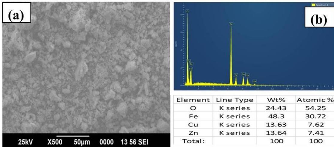
Fig.2. Images of Zinc copper ferrite nanoparticles annealed at 600°C (a) SEM (b) EDX analysis.
