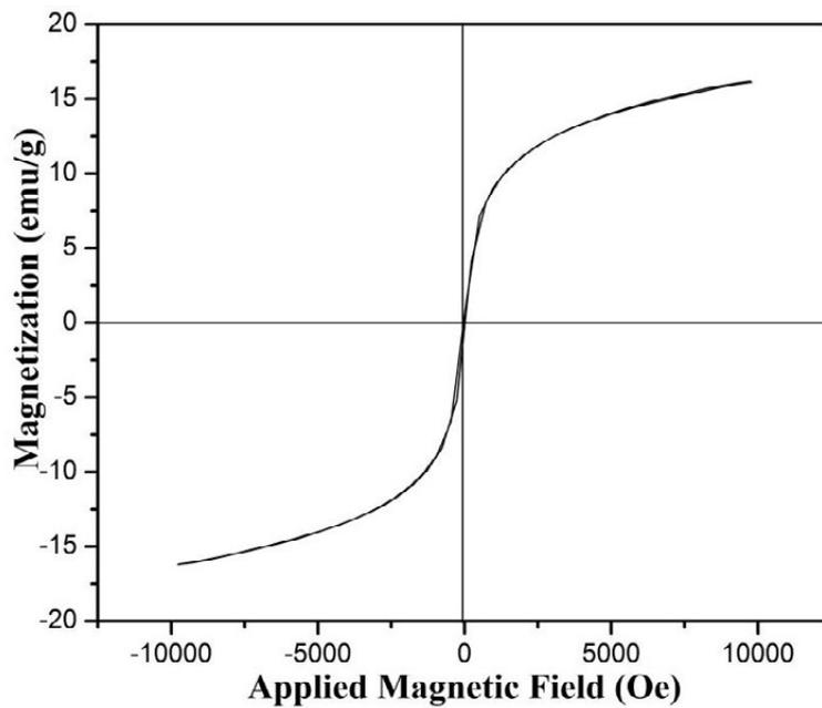
Fig.5. Magnetic hysteresis loops for Zinc copper ferrite nanoparticles annealed sample at 600°C.
