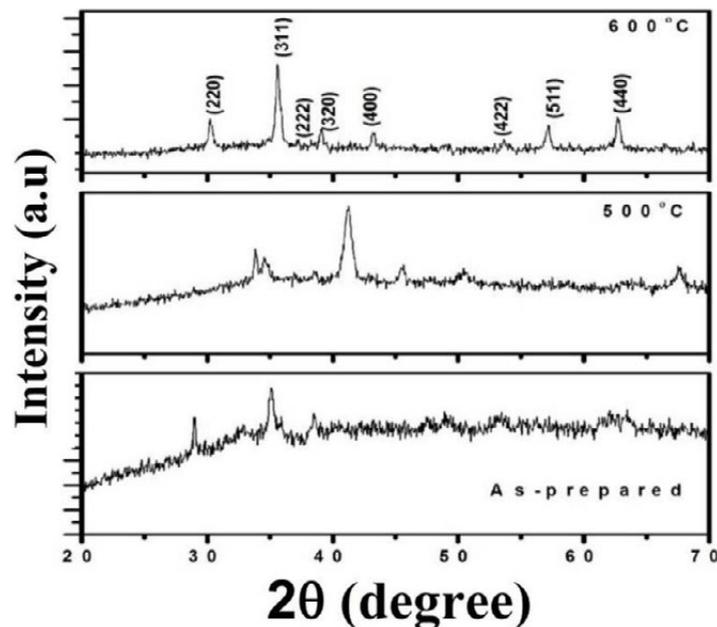
Fig.1. XRD patterns of Zinc copper ferrite nanoparticles as prepared, annealed at 500°C, and 600°C.
