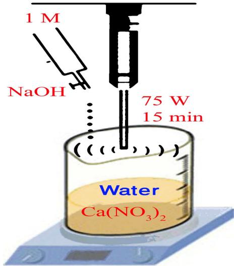
**Fig. 1.** Schematic diagram of preparation of Ca(OH)<sub>2</sub> nanoparticles.
