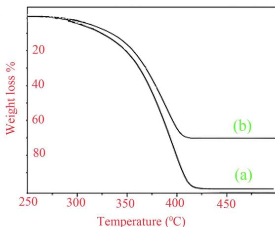
**Fig. 8.** TGA curves of (a) pure paraloid (b) paraloid-MWCNT-Ca(OH)<sub>2</sub> nanocomposite.
