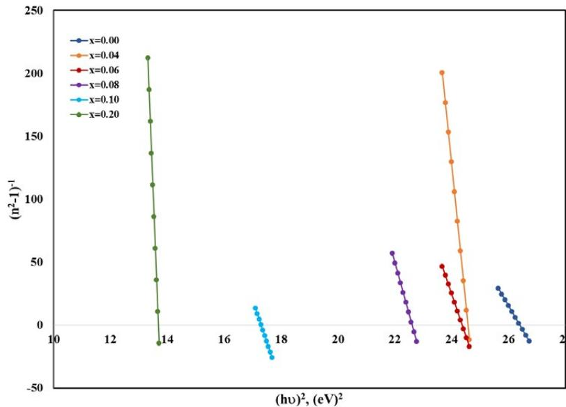
Fig. 10. Plots of (n<sup>2</sup>- 1)<sup>-1</sup> as a function of (hu)<sup>2</sup> for BaZr<sub>1-x</sub>Co<sub>x</sub>O<sub>3</sub> nanoparticles.
