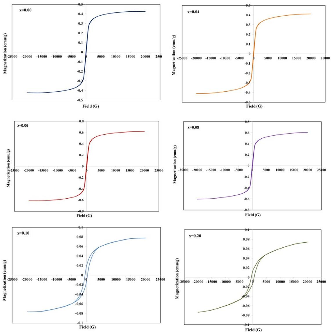
Fig. 13. Room temperature magnetic hysteresis loops ( $M$ - $H$ ) of BaZr<sub>1-x</sub>Co<sub>x</sub>O<sub>3</sub> nanoparticles,  $0.00 \leq x \leq 0.20$ .
