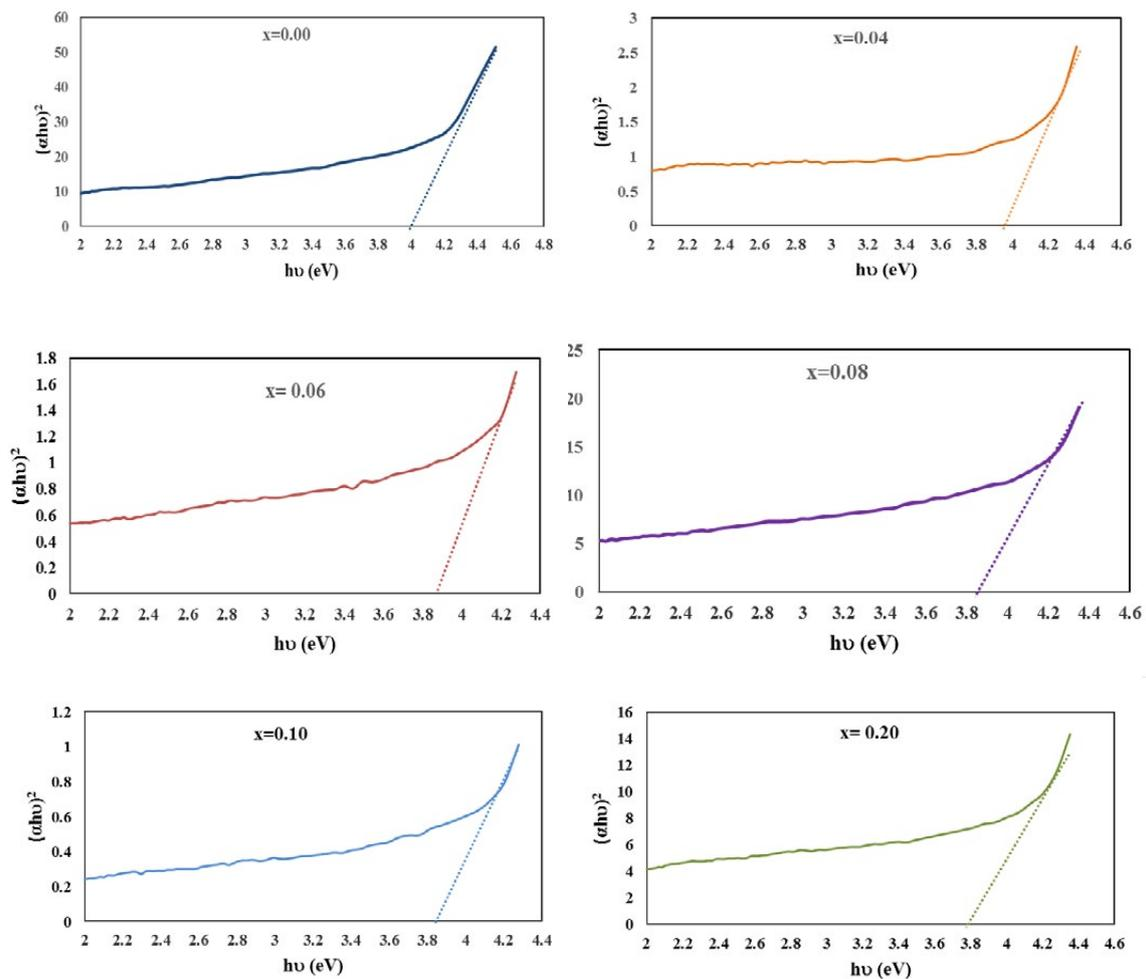
Fig. 8. Tauc plots of BaZr<sub>1-x</sub>Co<sub>x</sub>O<sub>3</sub> nanoparticles, 0.00 ≤ x ≤ 0.20.
