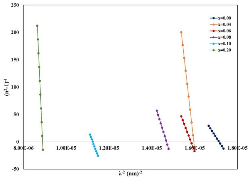
Fig. 11. Plots of  $(n^2 - 1)^{-1}$  as a function of  $\lambda^{-2}$  for BaZr<sub>1-x</sub>Co<sub>x</sub>O<sub>3</sub> nanoparticles.
