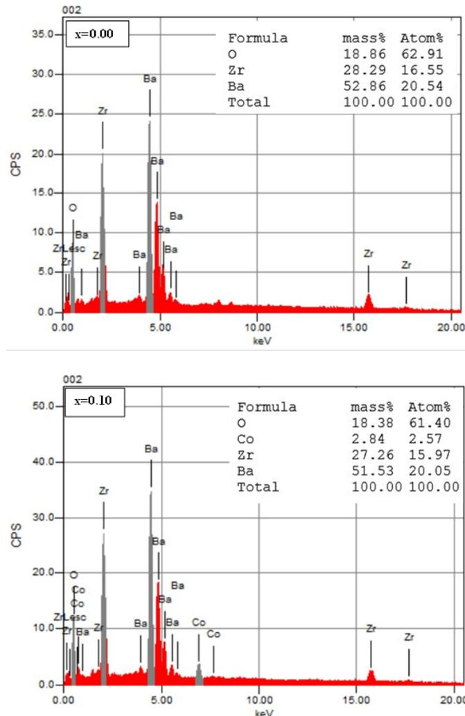
Fig. 5. EDS spectrum of BaZr<sub>1-x</sub>Co<sub>x</sub>O<sub>3</sub>, (a) x = 0.00, (b) x = 0.10.
