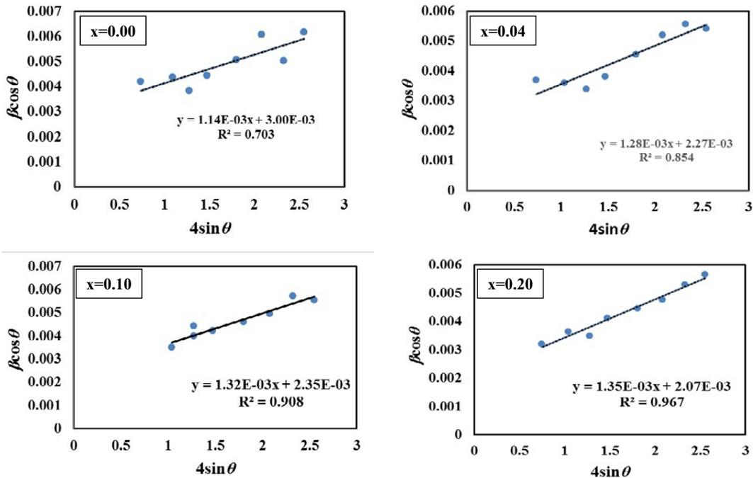
Fig. 3. Plots of  $\beta \cos \theta$  Vs.  $4 \sin \theta$  of BaZr<sub>1-x</sub>Co<sub>x</sub>O<sub>3</sub> nanoparticles, (a) x = 0.00, (b) x = 0.04 (c) x = 0.10 and (d) x = 0.20.
