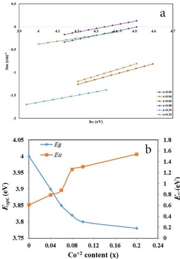
Fig. 9. a) Urbach plots of BaZr<sub>1-x</sub>Co<sub>x</sub>O<sub>3</sub> nanoparticles. b) The variation of optical band gap and Urbach energy with Co<sup>2+</sup> content (x).
