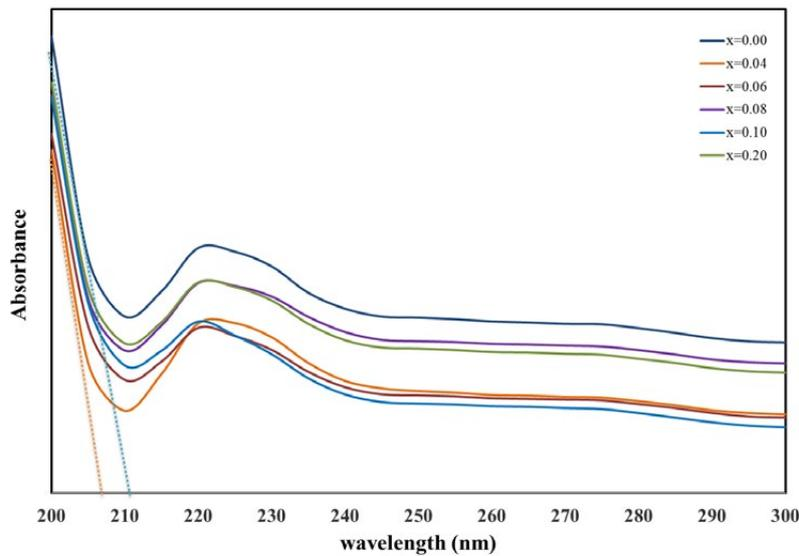
Fig. 7. UV absorption spectra of BaZr<sub>1-x</sub>Co<sub>x</sub>O<sub>3</sub> nanoparticles.
