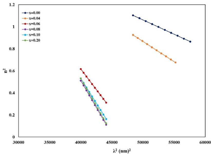
Fig. 12. Plots of  $n^2$  as a function of  $\lambda^2$  for BaZr<sub>1-x</sub>Co<sub>x</sub>O<sub>3</sub> nanoparticles.
