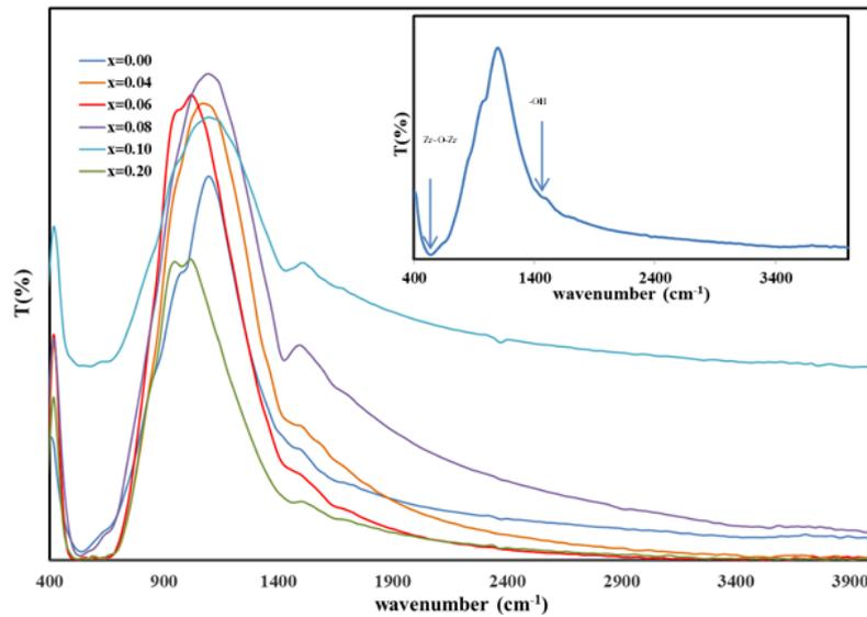
Fig. 6. FT-IR spectra of BaZr<sub>1-x</sub>Co<sub>x</sub>O<sub>3</sub> nanoparticles, 0.00 ≤ x ≤ 0.20.
