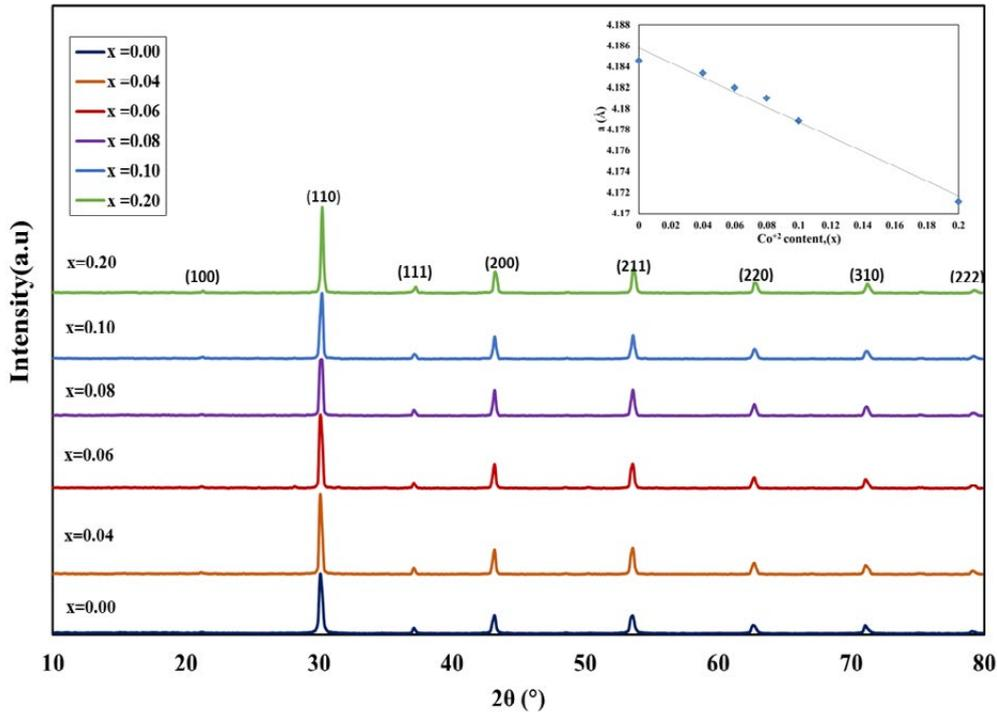
Fig. 1. XRD patterns of BaZr<sub>1-x</sub>Co<sub>x</sub>O<sub>3</sub> nanoparticles, 0.00 ≤ x ≤ 0.20. The inset shows the variation of unit cell parameter (a) with Co<sup>2+</sup> content, x for BaZr<sub>1-x</sub>Co<sub>x</sub>O<sub>3</sub> nanoparticles.
