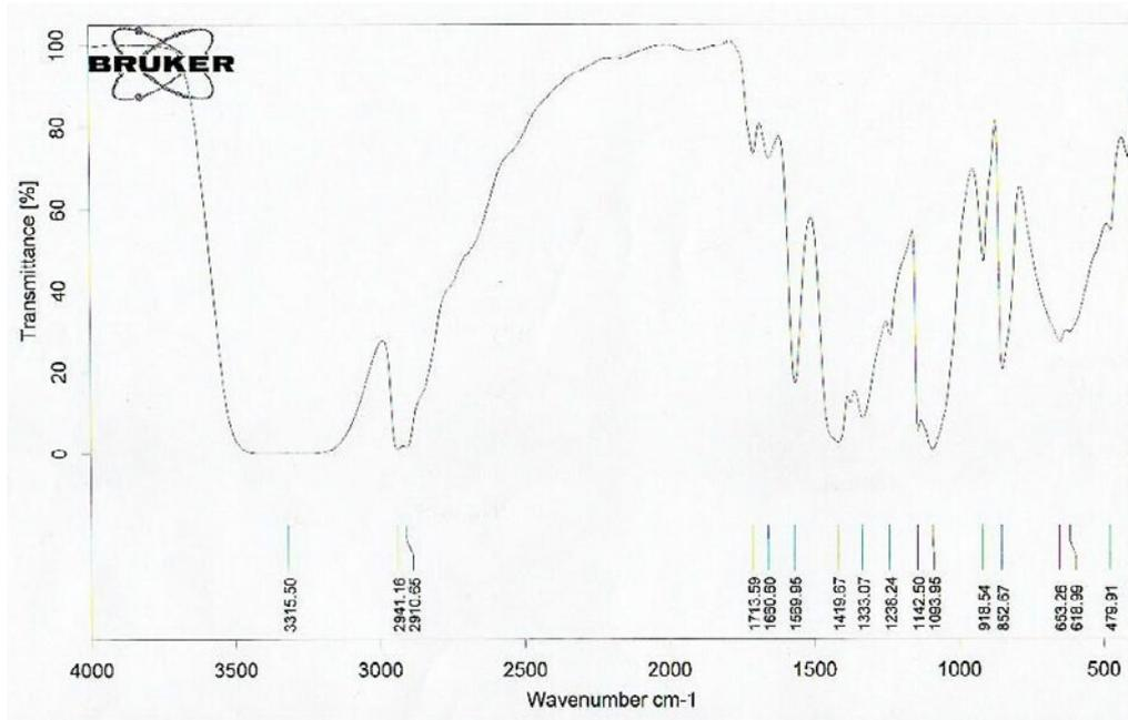
Fig. 10. FT-IR spectrum of Poly vinyl alcohol
