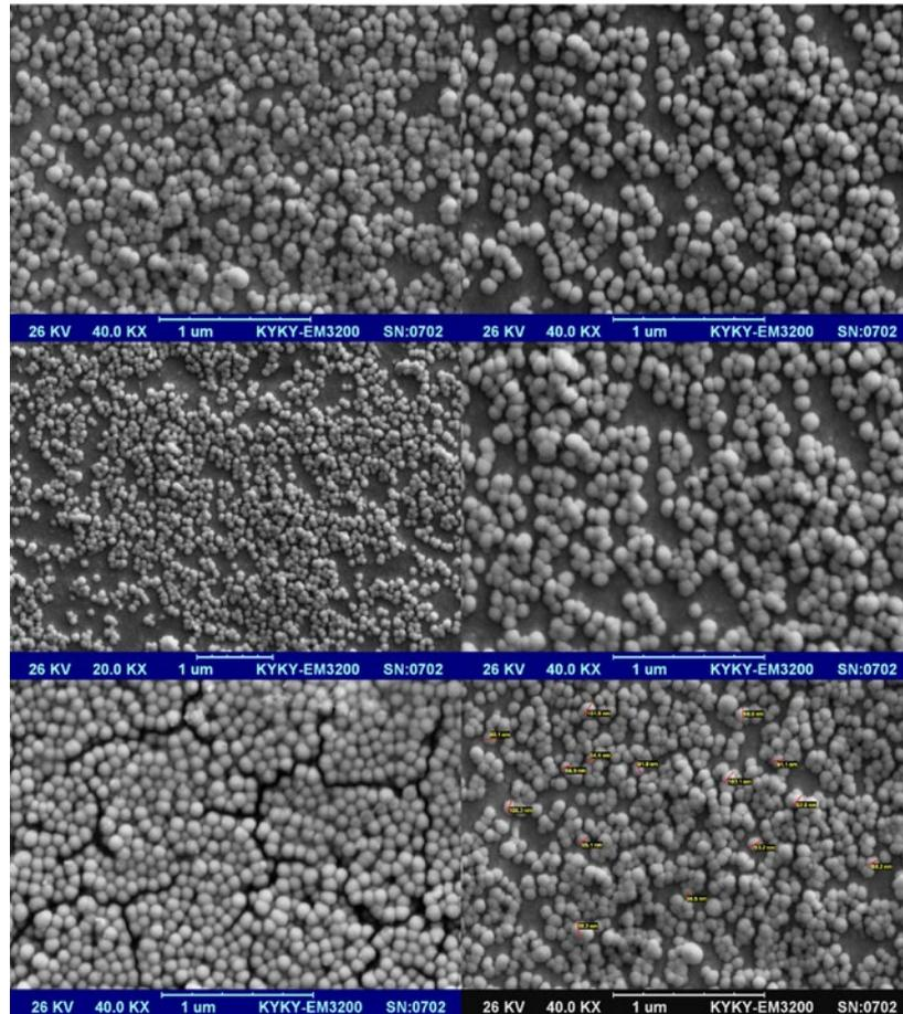
Fig. 6. SEM images of COFe<sub>2</sub>O<sub>4</sub> nanoparticles with ethylene glycol solvent and heating time of 5 minutes
