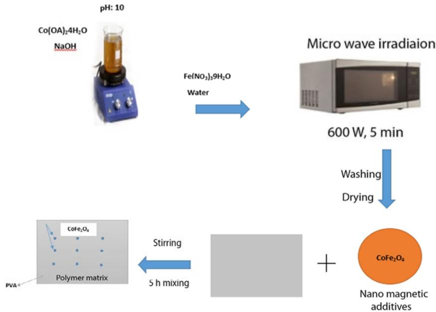
Fig.1. Schematic of samples including Cobalt ferrite and polyvinyl alcohol nanocomposite preparation.
