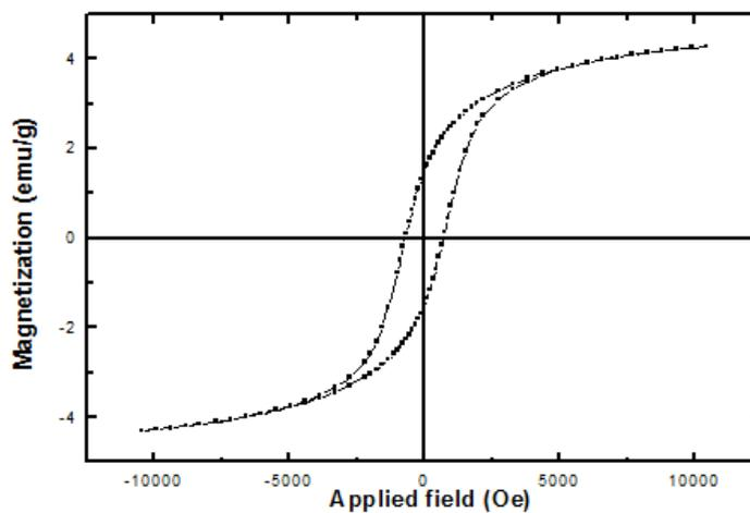
Fig. 9. VSM curve of PVA- CoFe<sub>2</sub>O<sub>4</sub> nanocomposite
