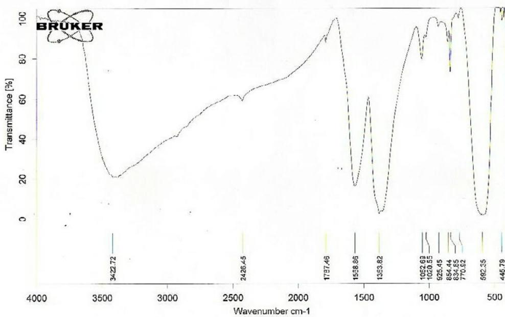
Fig. 11. FT-IR spectrum of CoFe<sub>2</sub>O<sub>4</sub>-PVA nanocomposite
