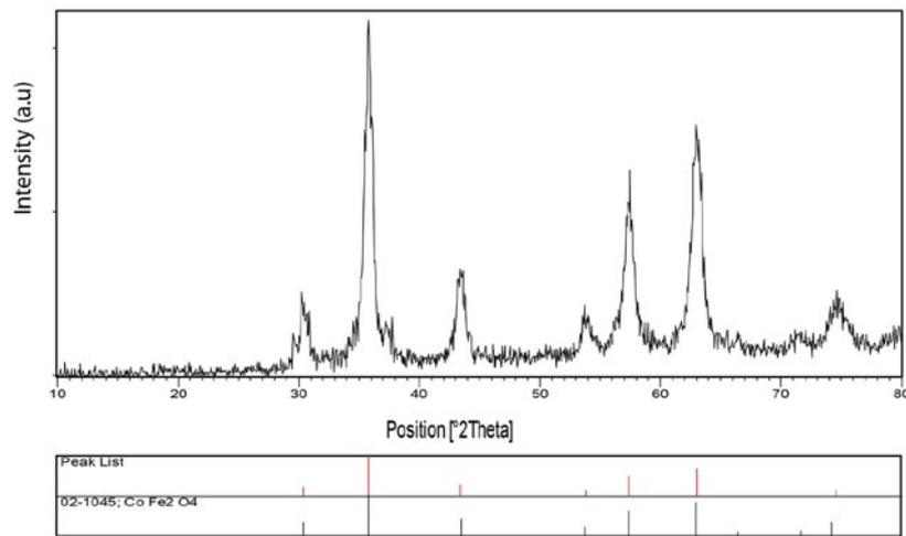
Fig. 2. XRD pattern of  $\text{CoFe}_2\text{O}_4$  nanoparticles
