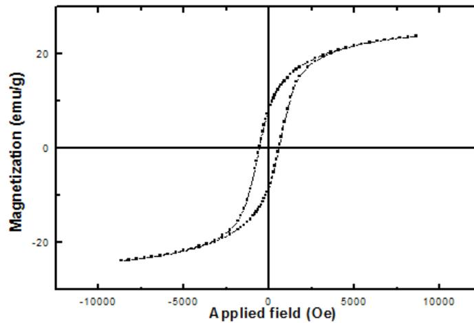
Fig. 8. VSM curve of CoFe<sub>2</sub>O<sub>4</sub> nanoparticles
