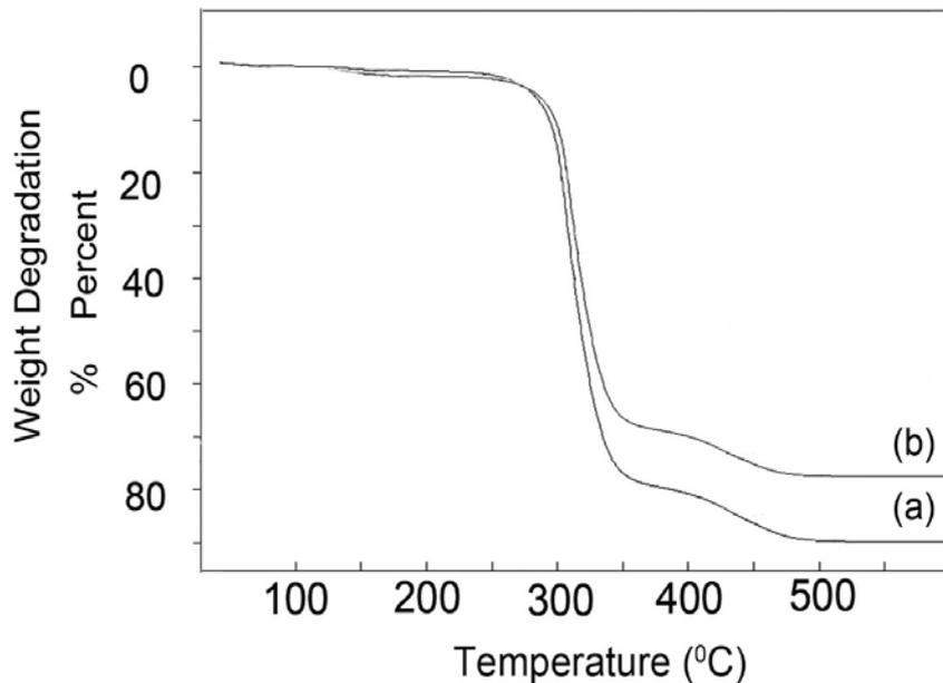
Fig. 12. Thermal resistance graph of CoFe<sub>2</sub>O<sub>4</sub>- PVA nanocomposites (a) and PVA polymer (b)
