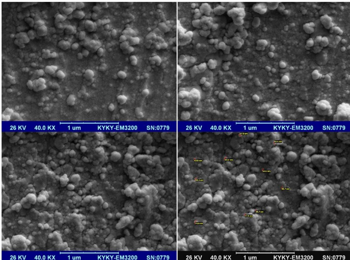
Fig. 5. SEM images of  $\text{CoFe}_2\text{O}_4$  nanoparticles with combination solvent (90% water, 10% ethylene glycol) and heating time of 5 minutes
