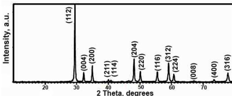
Fig. 2. XRD patterns of CdMoO<sub>4</sub> nanostructures
