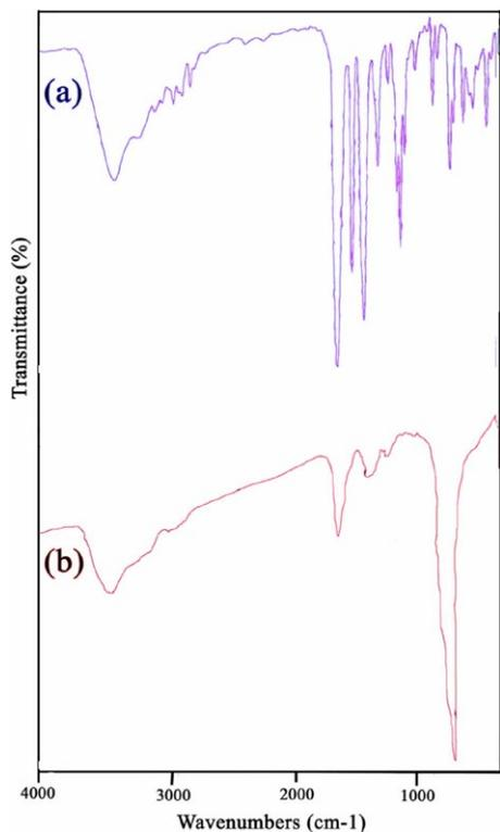
Fig. 1. FT-IR spectra of: (a) Cd(Sal)<sub>2</sub>, (b) CdMoO<sub>4</sub> nanostructures
