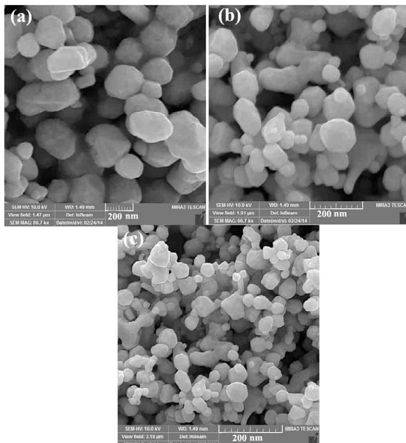
Fig. 7. SEM images of sphere-like CdMoO<sub>4</sub> nanostructures gained from Cd(Sal)<sub>2</sub> and Na<sub>2</sub>MoO<sub>4</sub>·2H<sub>2</sub>O in water via sonochemical approach in:(a) 200 ,(b) 300 and (c) 400 W in 20 min.
