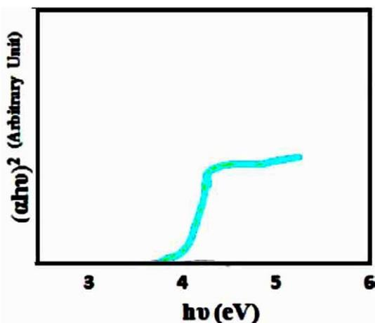
Fig. 4. The  $(\alpha h\nu)^2$  vs  $h\nu$  plot of CdMoO<sub>4</sub> nanostructures.
