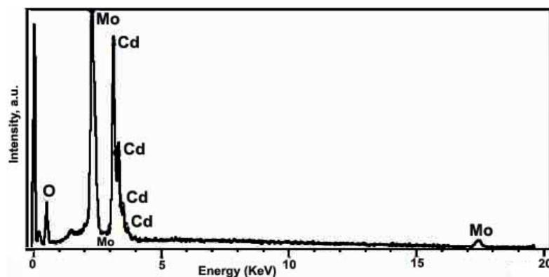
Fig. 3. EDX pattern of CdMoO<sub>4</sub> nanostructures
