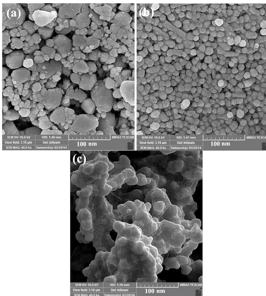
Fig. 6. SEM images of CdMoO<sub>4</sub> nanostructures gained from Cd(Sal)<sub>2</sub> and Na<sub>2</sub>MoO<sub>4</sub>·2H<sub>2</sub>O via sonochemical approach with different surfactants:(a) CTAB (b) PVP and (c) SDS in 400W and 20 min.
