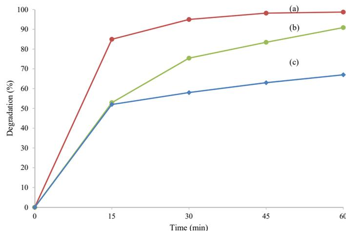
Fig. 3. The degradation of the dyes by the ZnO/ACn prepared by (a) solid-state, (b) precipitation method and commotional Degusa TiO<sub>2</sub> against methyl orange
