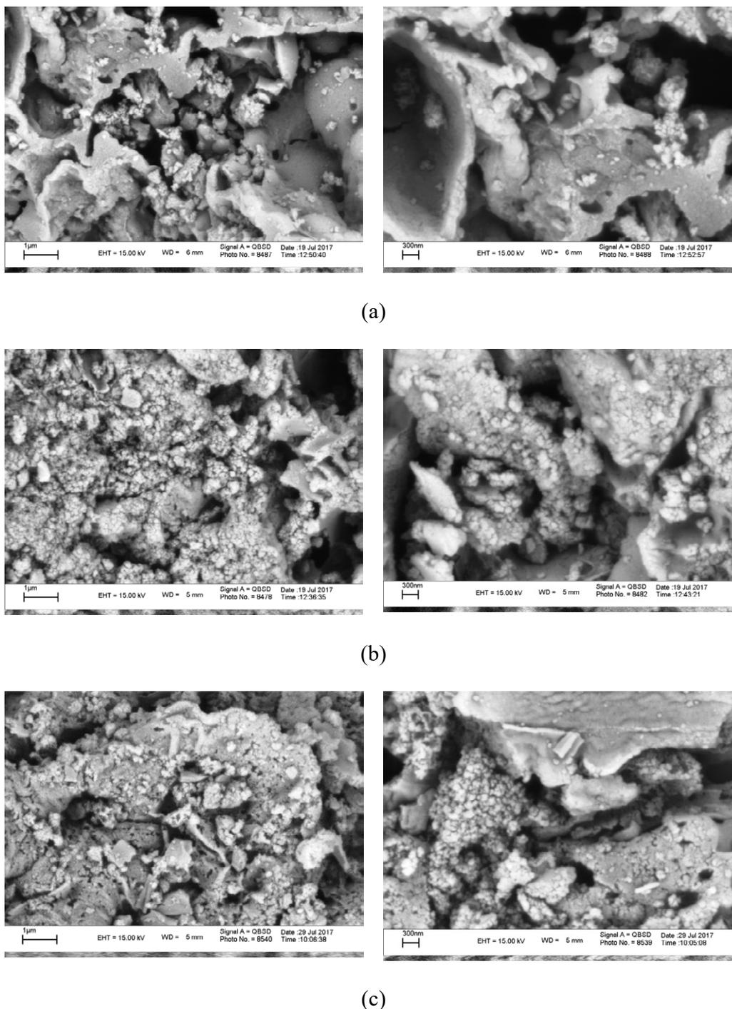
Fig. 1. The SEM micrographs of (a) activated carbon and ZnO/ACn prepared by (b) solid-state and (c) precipitation method.
