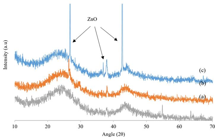
Fig. 2. The XRD patterns of (a) activated carbon and ZnO/ACn prepared by (b) solid-state and (c) precipitation method.
