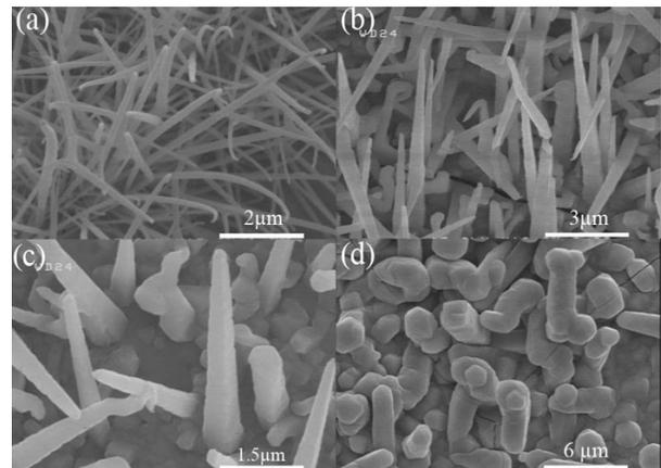
**Fig. 5.** SEM images of GeNWs with different ratio of Ar and H<sub>2</sub> as carrier gas.
