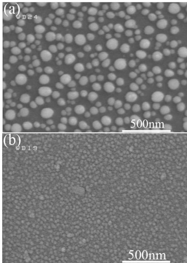
**Fig. 3.** SEM images of Au nanoparticles from (a) Au thin layer after annealing process at 500 °C and (b) Au colloidal solution.
