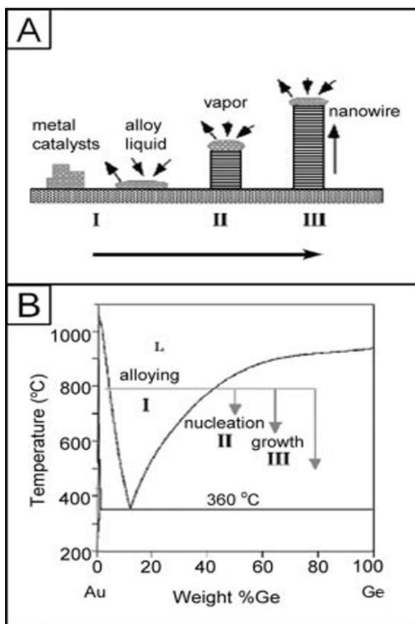
**Fig. 1.** (a) The VLS mechanism of nanowires growth through catalyst seeds and (b) the binary phase diagram of Ge and Au [25].
