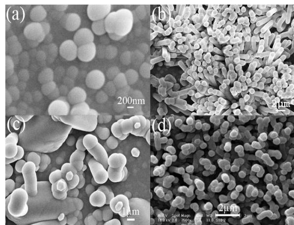
**Fig. 2.** SEM images of samples (a-c) with Au thin film catalyst for different gas flows: 60, 80, 100 sccm, and (d) with Au colloidal solution catalyst for 80 sccm.
