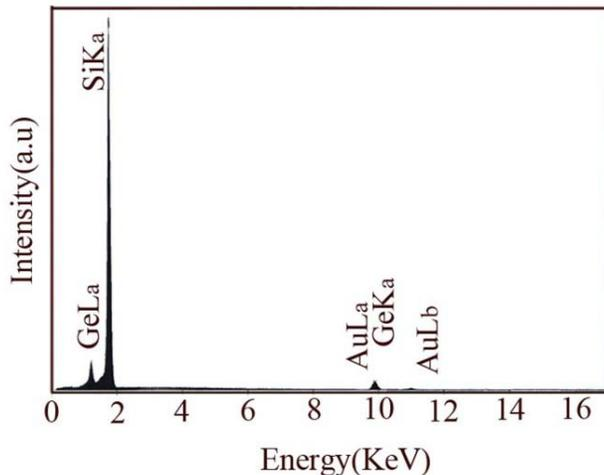
**Fig. 4.** EDS spectrum of the GeNWs with 80 sccm as carrier gas flow and catalyst of Au colloidal solution.
