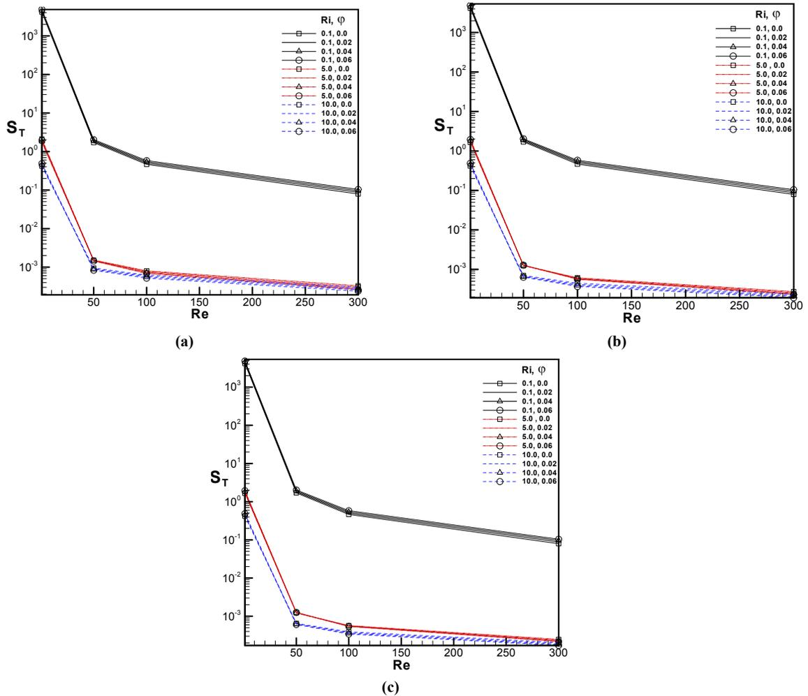
Fig. 4. Total values of entropy generation for (a)  $\gamma=-90^\circ$ , (b)  $\gamma=-0^\circ$  and (c)  $\gamma=90^\circ$ .
