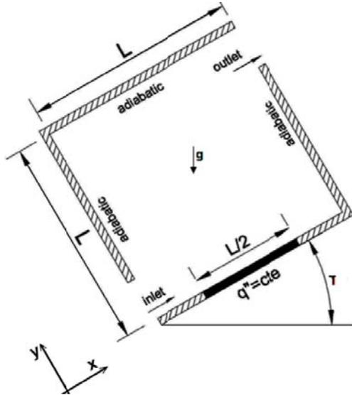
Fig. 1. Schematic of the cavity.
