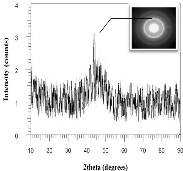
**Fig. 3.** XRD Pattern of Iron nanoparticles Synthesis.
