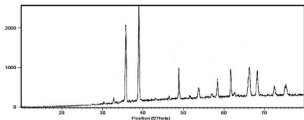
Fig. 1. The XRD pattern of copper(II) oxide nanoparticles.
