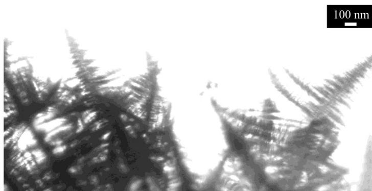
Fig. 6. TEM image of Pd dendrite nanostructures.
