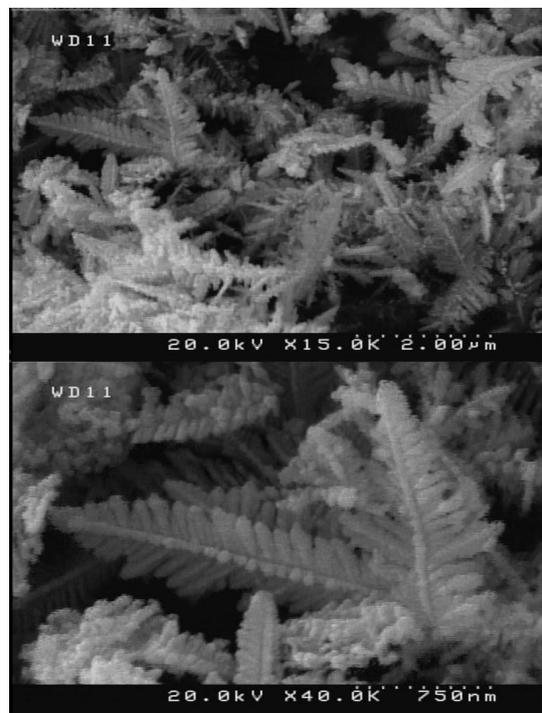
Fig. 9. SEM images of Ag synthesized at 160 °C for 10 h
