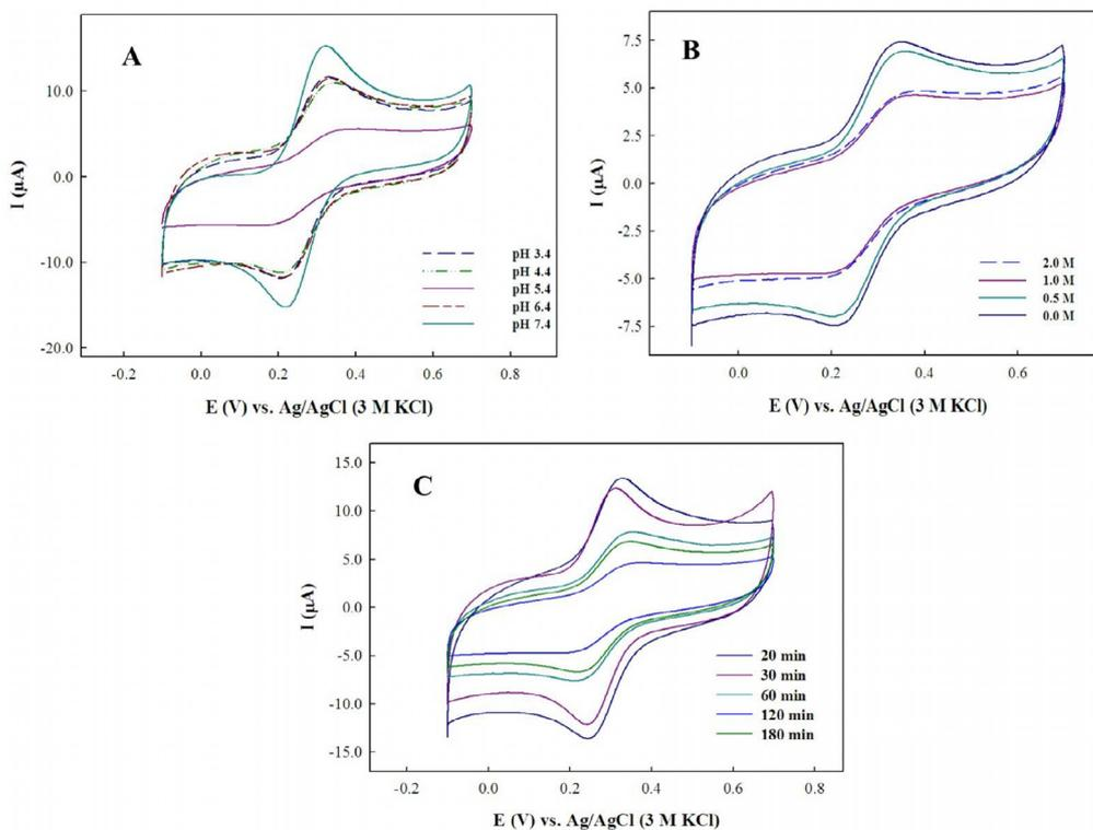
Fig. 5. Cyclic voltammograms recorded in presence of 0.01 M  $[\text{Fe}(\text{CN})_6]^{3-/4-}$  containing 0.1 M KCl for ss-DNA immobilization on MWCNT-COOH/GCE as a function of (A) pH, (B) NaCl concentration and (C) incubation time.
