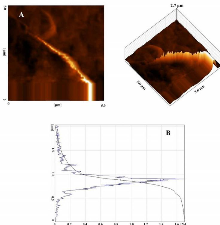
Fig. 6. (A) Typically AFM image of MWCNT-COOH (image size:  $5\mu\text{m} \times 5\mu\text{m} \times 2.7\mu\text{m}$ ), (B) Image height distribution.
