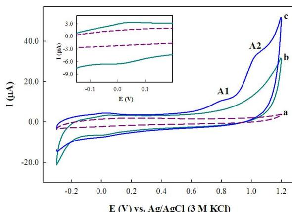
Fig. 2. Cyclic voltammograms of the modified GCE recorded in PBS (pH 7.0) at a scan rate of 0.1 Vs<sup>-1</sup>, in the potential range between -0.3 to +1.2 V (a) bare GCE, (b) MWCNT-COOH/GCE, and (c) ss-DNA/MWCNT-COOH/GCE.
