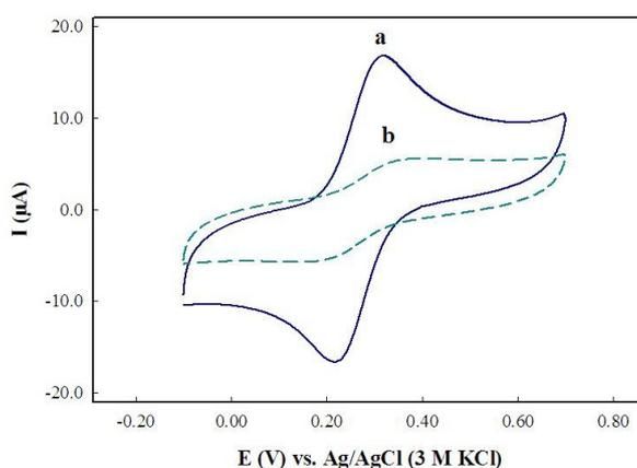
Fig. 3. Cyclic voltammograms of (a) MWCNT-COOH/GCE and (b) ss-DNA/MWCNT-COOH/GCE in presence of 0.01 M [Fe(CN)<sub>6</sub>]<sup>3-/4-</sup> in 0.1 M KCl. Scan rate: 0.1 Vs<sup>-1</sup>.
