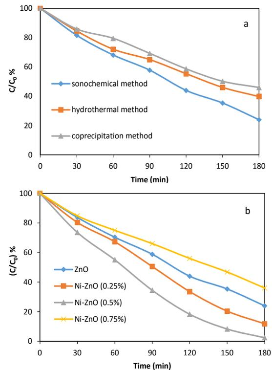
Fig. 8. Photodegradation of methyl orange (MO) using the samples: (a) ZnO samples (different methods), (b) Ni-ZnO NPs (sonochemical method).
