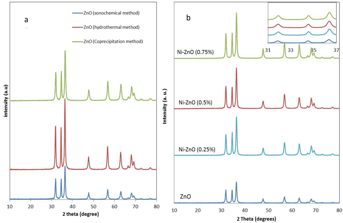
Fig. 4. XRD spectra of samples: (a) ZnO samples (different methods), (b) Ni-ZnO NPs (sonochemical method).
