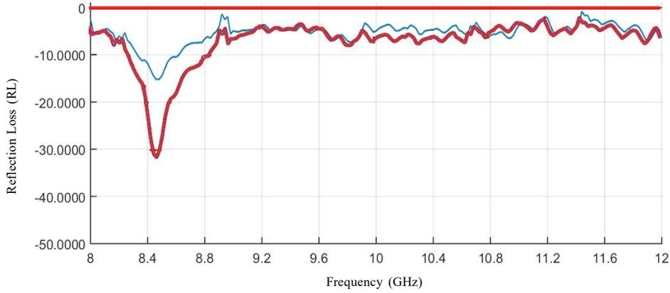
Fig. 8. The RL curve of A7 (blue) and A8 (red) samples.
