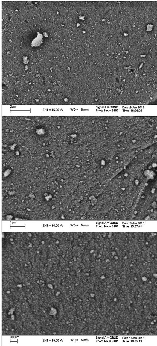
Fig. 3. SEM images of CoFe<sub>2</sub>O<sub>4</sub> nanoparticles at 400 ml of water (diluted sample)
