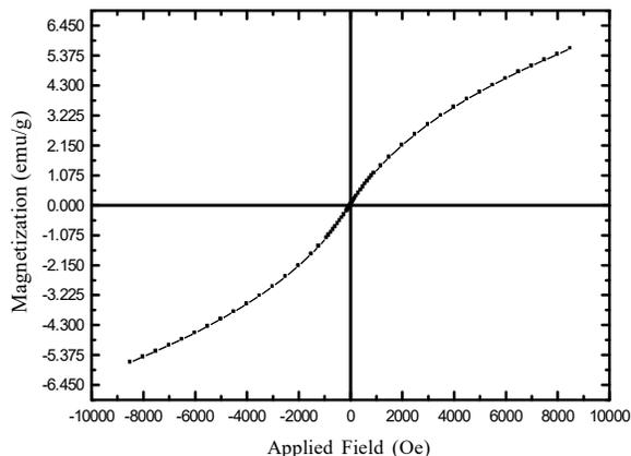
Fig. 8. AGFM of  $\text{CoFe}_2\text{O}_4$  nanoparticles.
