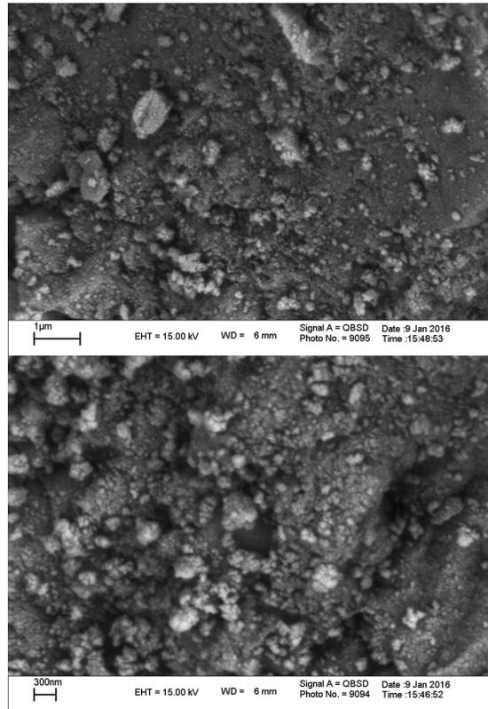
Fig. 4. SEM image of ferrite nanoparticles obtained by gelatin
