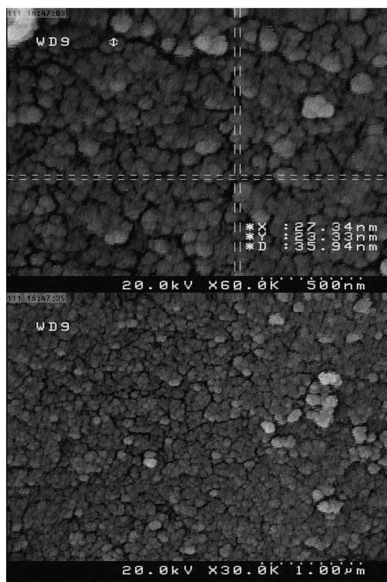
Fig. 2. SEM images of surfactant-free  $\text{CoFe}_2\text{O}_4$  nanoparticles
