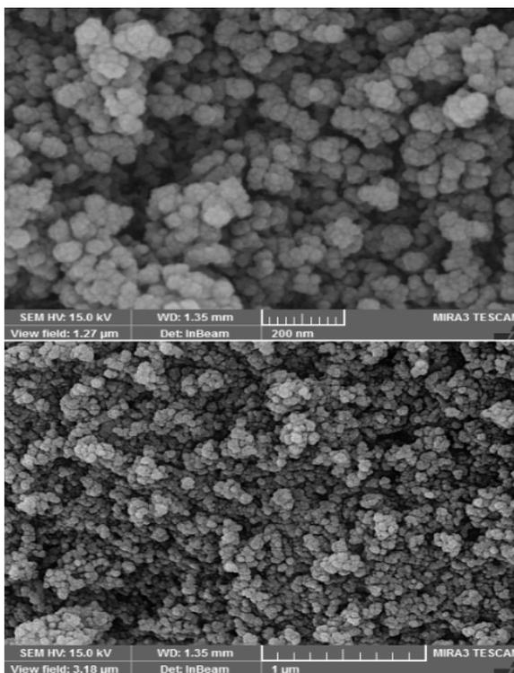
Fig. 3. SEM images of CoFe<sub>2</sub>O<sub>4</sub> stabilized by SDBS
