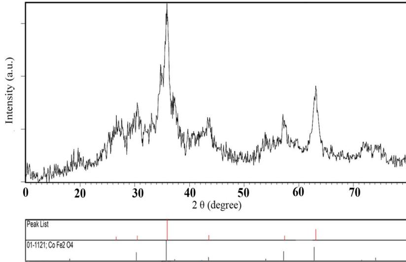
**Fig. 1.** XRD patterns for CoFe<sub>2</sub>O<sub>4</sub> synthesized by hydrothermal method.
