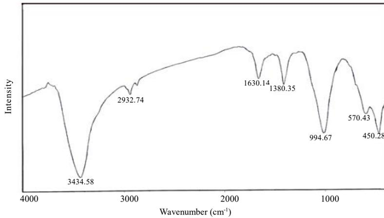
**Fig. 2.** IR spectrum for CoFe<sub>2</sub>O<sub>4</sub> synthesized by hydrothermal method
