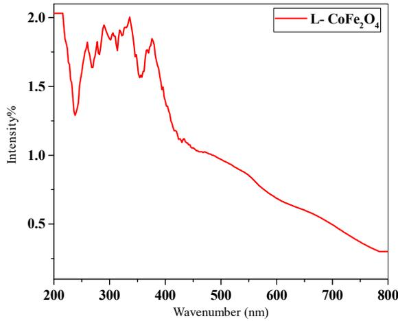
Fig. 6. UV-vis spectrum (DRS) for 2-hydroxyacetophenone-CoFe<sub>2</sub>O<sub>4</sub> nanoparticle.
