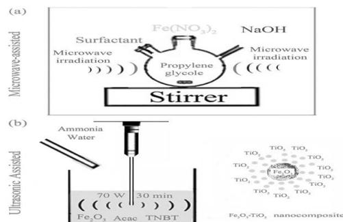
Fig. 1. Schematic of (a) microwave (b) ultrasonic
