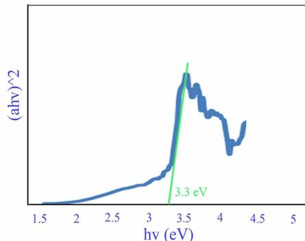
**Fig. 9.** Diffuse reflectance spectroscopy analysis of Fe<sub>2</sub>O<sub>3</sub>-TiO<sub>2</sub> nanoparticles
