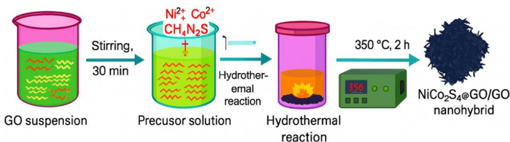
Fig. 1. Synthesis process of NiCo 2 S 4 @rGO.
