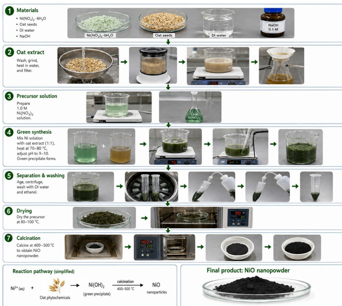
Fig. 1. Schematic illustration of the complete synthesis protocol for NiO nanoparticles using oat seed extract, showing the seven sequential steps from raw materials through calcination to the final black NiO nanopowder, along with the overall reaction pathway.
