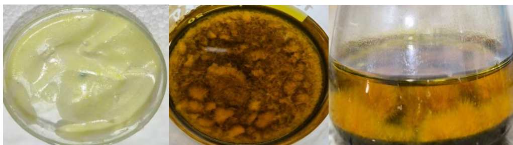
Fig. 4. Crystallization of the polyamide/CQDs nanocomposite during solvent evaporation.
