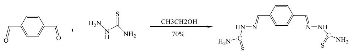
Terephthalaldehyde Thiosemicarbazide Terephthalaldehyde bis(thiosemicarbazone) Fig.1. Synthesis pathways of Schiff-base diamine monomer: (A) Terephthalaldehyde bis(thiosemicarbazone) (TBT).
