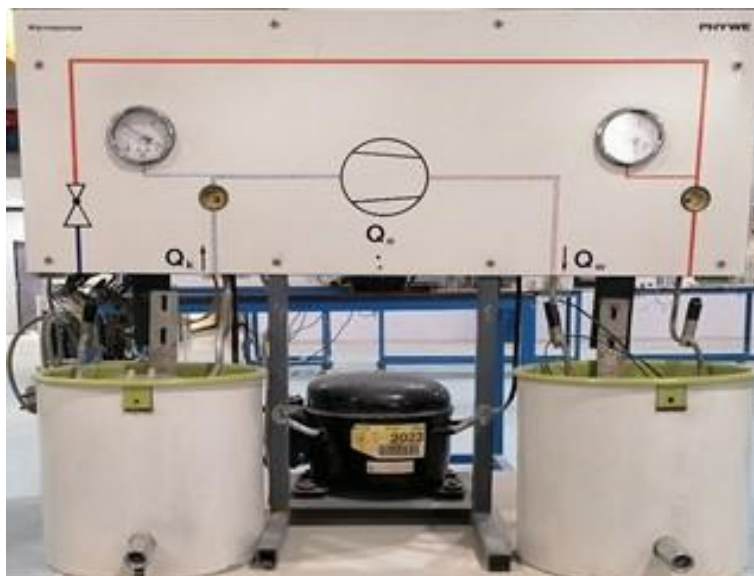
Fig. 3. A heat pump system device.
