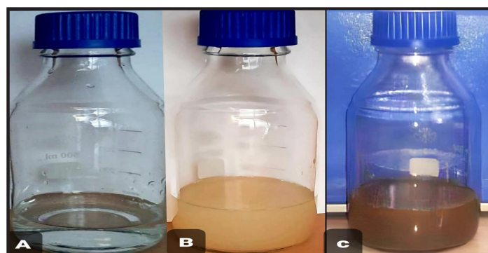
Fig. 1. Culture bottles containing (A) \text{AgNO}_3 , (B) fenugreek seed extract without \text{AgNO}_3 and (c) Mixture of fenugreek seed extract with 1Mm \text{AgNO}_3 after incubation for 24hrs.
