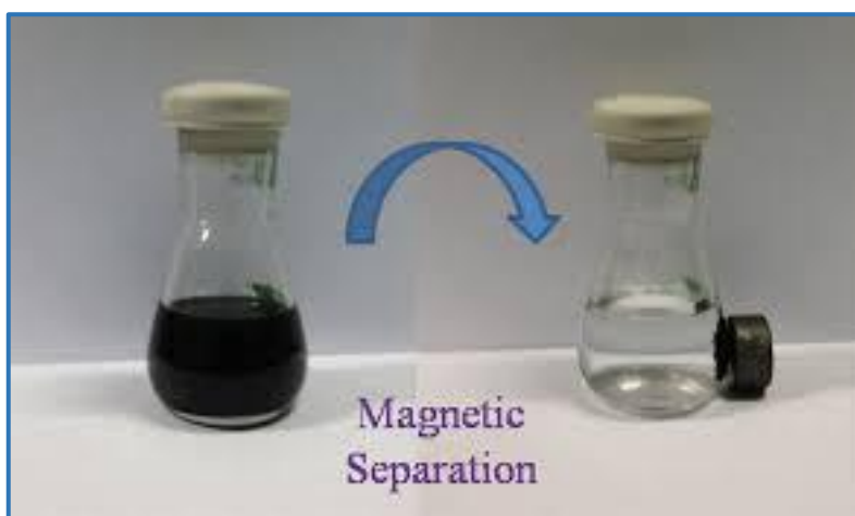
Fig. 2. Magnetic separation of \text{Fe}_3\text{O}_4\text{@NCs}/\text{TiCl} .
