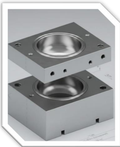
Fig. 2. Stainless-steel die, 3 cm in internal diameter, used for cold compaction of the composite discs.
