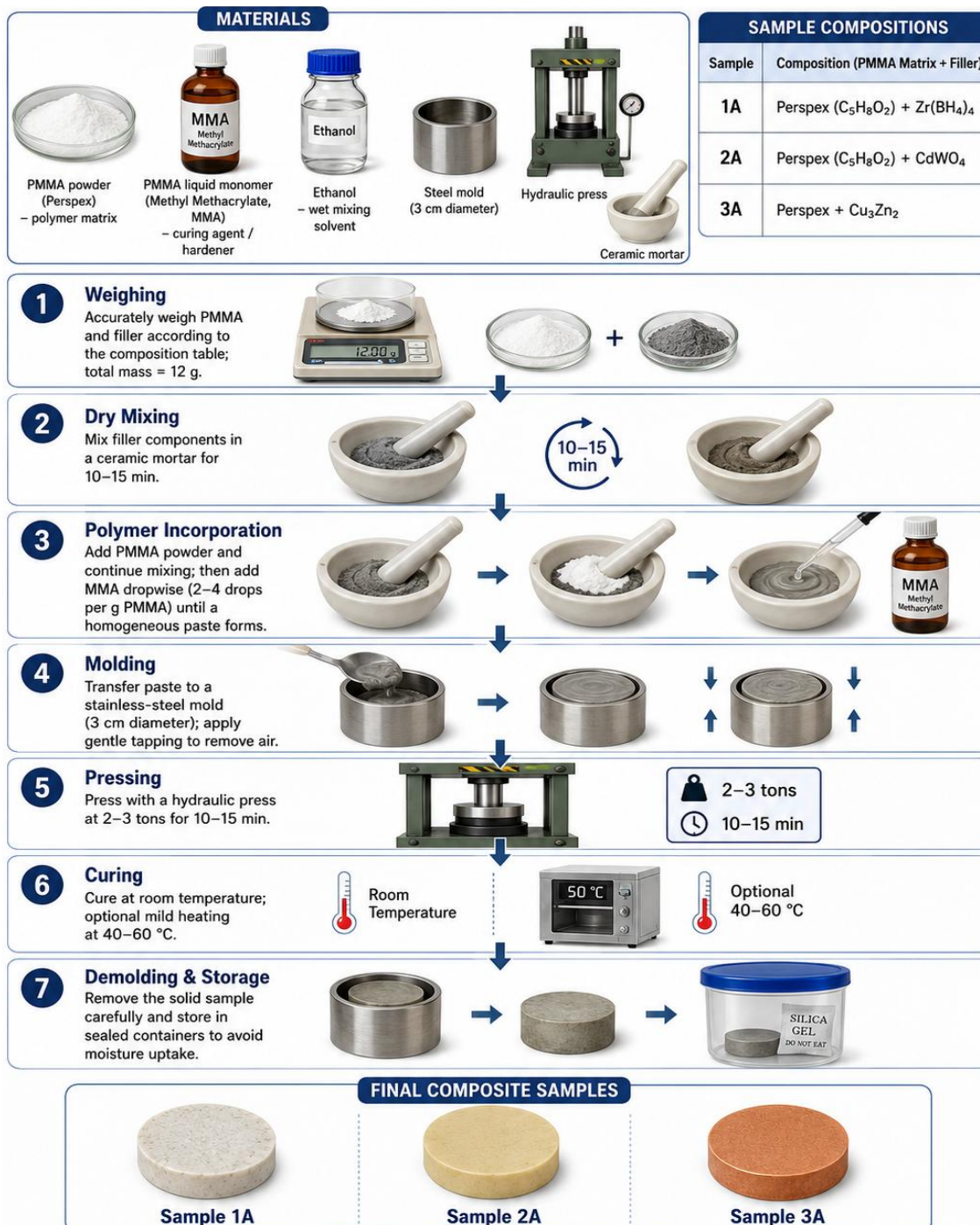
Fig. 3. Flow chart of the fabrication route of the PMMA-based composites, from weighing of the constituents through dry mixing, MMA-assisted polymer incorporation, moulding, uniaxial pressing, curing and demoulding, together with the compositions of the three sample groups.
