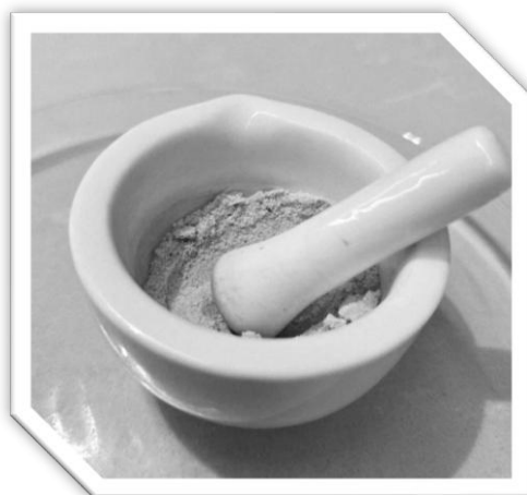
Fig. 1. Agate/ceramic mortar and pestle used for the dry homogenization of the filler powders prior to polymer incorporation.
