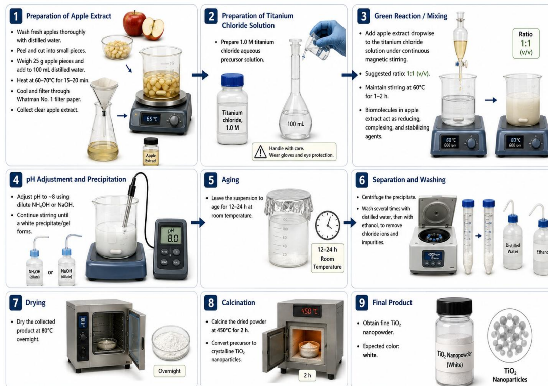
Fig. 1. Schematic overview of the green synthesis of TiO 2 nanoparticles using red apple ( Malus domestica ) extract: preparation of the extract, mixing with the 1.0 M TiCl 4 precursor, pH adjustment, aging, washing, drying, and calcination at 450 °C.
