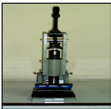
A B Fig. 1. A - Manual cutter for cutting samples. B – Test samples after cutting.
