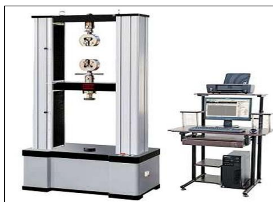
Fig. 2. A measuring device for examining tensile properties, modulus of elasticity, and elongation.
