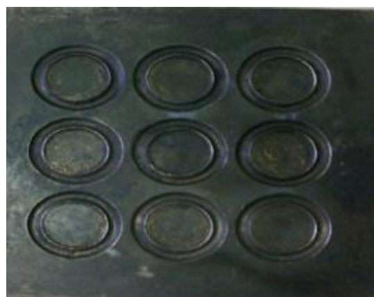
Fig. 3. Mold for producing hardness test samples.
