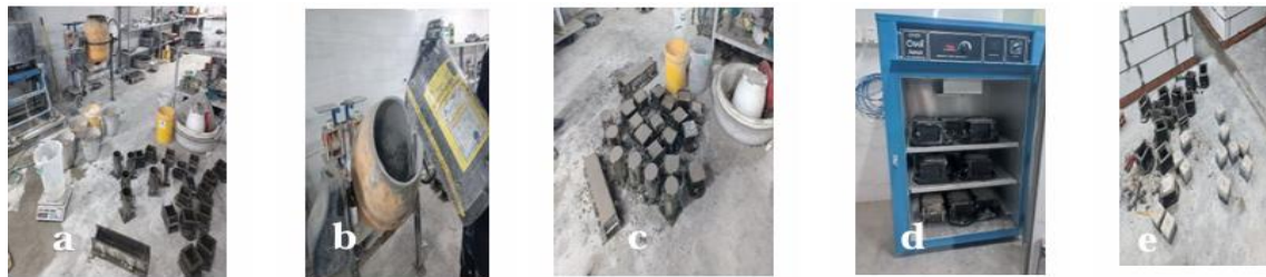
Fig. 3. illustrates the specimen preparation procedure, including (a) materials, (b) alkaline liquid mixing, (c) casting, (d) curing, and (e) demoulded specimens.
