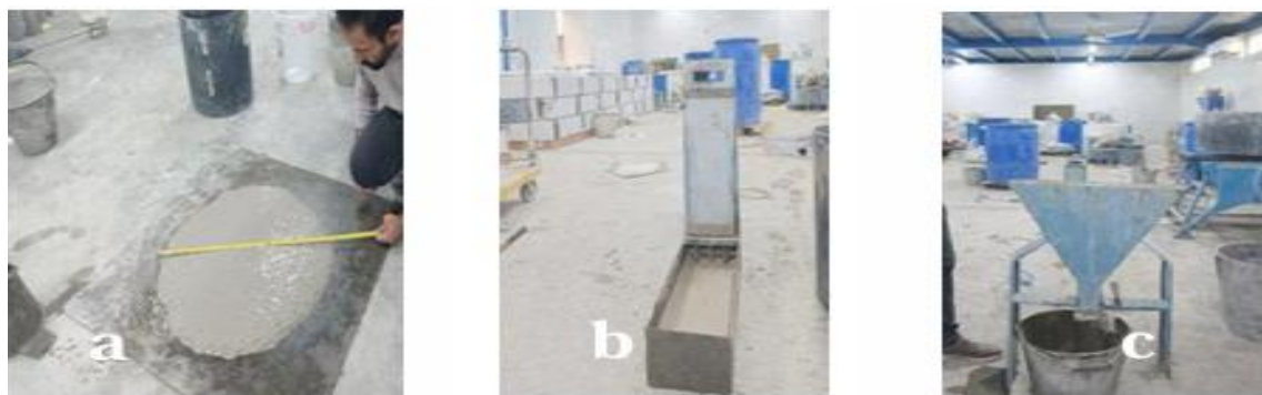
Fig. 8. Fresh Tests: a. Slump Flow, b. L-Box, and c. V-Funnel Flow.
