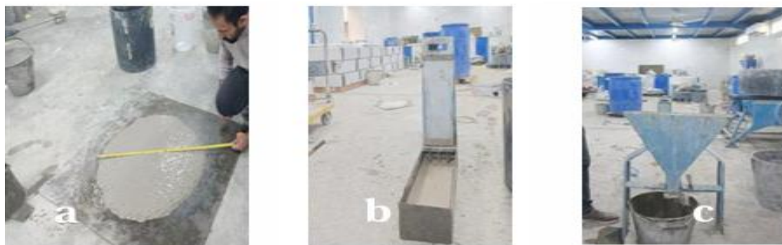
Fig. 7. Tests of Fresh Properties: a. Slump Flow Test, b. L-Box test, and C. V-Funnel Flow Time.
