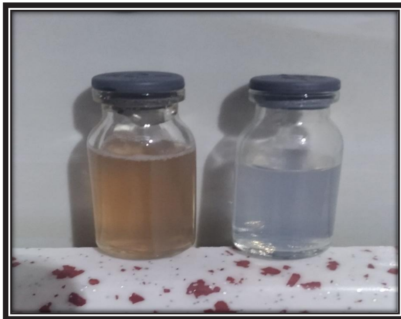
Fig. 1. Color change of silver nitrate solution (2 molar) After adding the aqueous extract of rosemary leaves.
