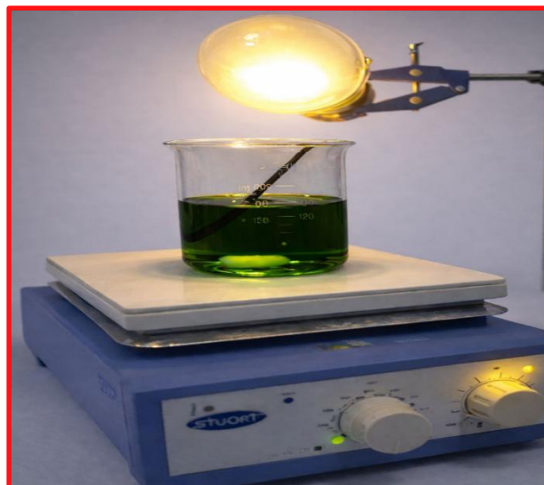
Fig. 2. Malachite green dye degradation by photo catalysis using the system of the photocatalytic cell.
