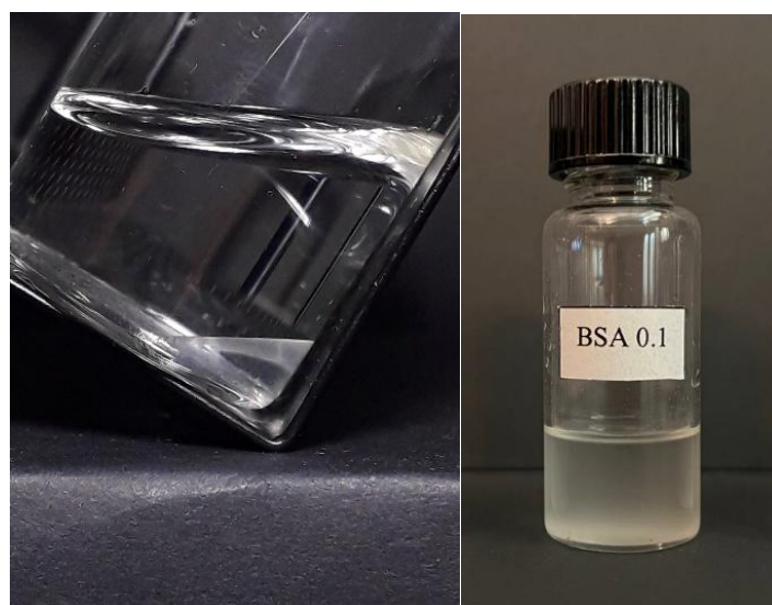
Fig. 5. The illustration of the two phase solution post-mixing (right side) and following emulsification and phase separation (left side).
