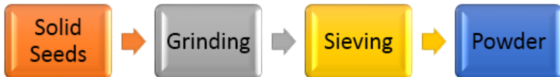
Fig. 3. Producing phases of Phoenix Dactylifera L. (Barhee) nano powder.
